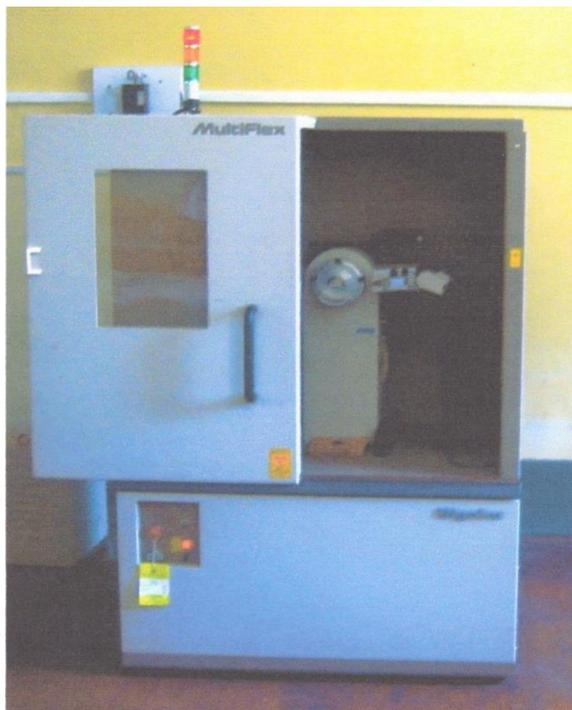
**Figure 3:** Photograph of the RIGAKU MULTIFLEX X-ray Diffractometer
