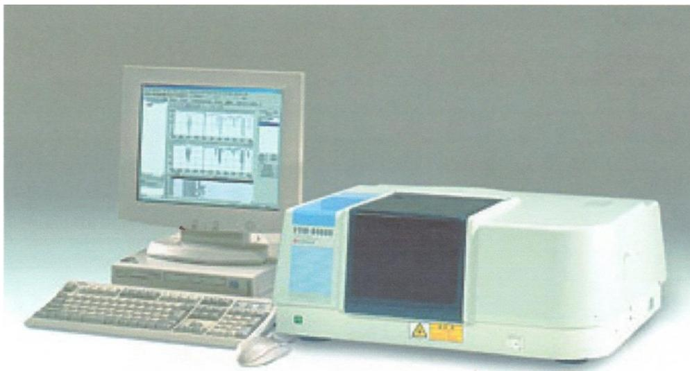
**Figure 4:** Photograph of the SHIMADZU FT IR-8400 Spectrophotometer
