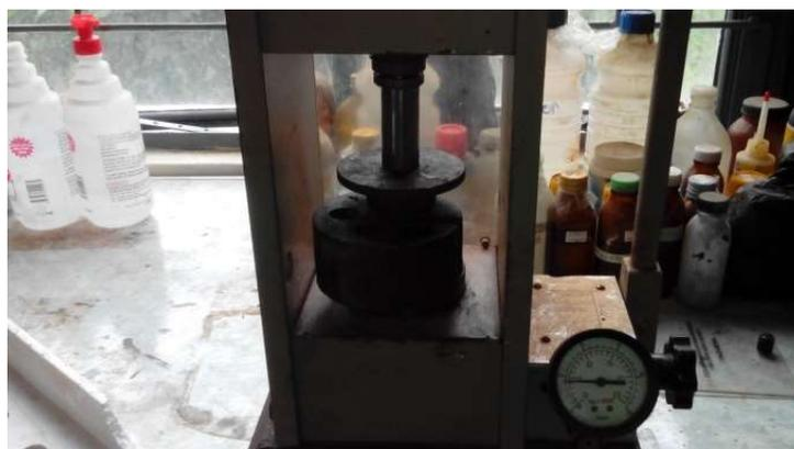
**Figure 2.** Photograph of SPECAC hydraulic pellet maker
