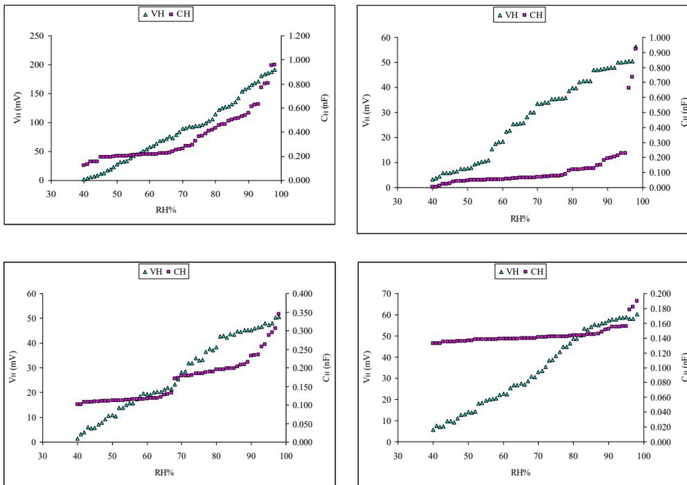
**Figure 5.** Plots of the variation of dc voltage  $V_H$  and capacitance  $C_H$  with relative humidity RH% of (c)  $Ni_{0.97-x}Zn_xCo_{0.03}Fe_2O_4$  where  $x = 0.75$  and (d) pure  $NiFe_2O_4$ , (e)  $CoFe_2O_4$  and (f)  $ZnFe_2$
