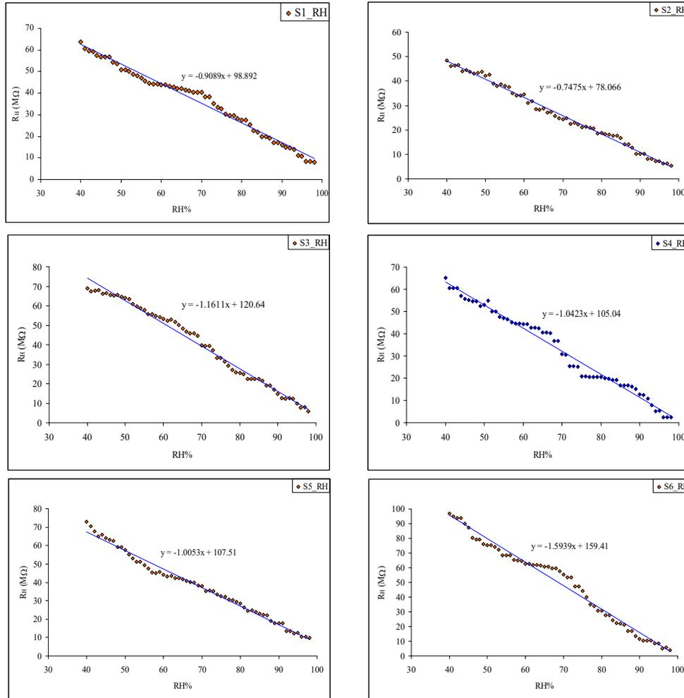
**Figure 4.** Plots of the variation of electrical resistance  $R_H$  with relative humidity RH% of  $Ni_{0.97-x}Zn_xCo_{0.03}Fe_2O_4$  where (a)  $x = 0.25$ , (b)  $x = 0.50$ , (c)  $x = 0.75$  and (d) pure  $NiFe_2O_4$ , (e)  $CoFe_2O_4$  and (f)  $ZnFe_2O_4$
