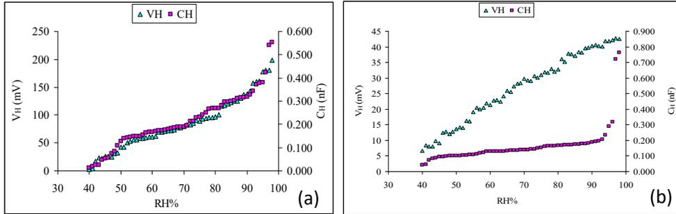
**Figure 5.** Plots of the variation of dc voltage  $V_H$  and capacitance  $C_H$  with relative humidity RH% of  $Ni_{0.97-x}Zn_xCo_{0.03}Fe_2O_4$  where (a)  $x = 0.25$  and (b)  $x = 0.50$
