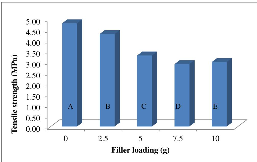
**Figure 6:** Tensile strength of natural rubber latex chitosan composites (A-E)
