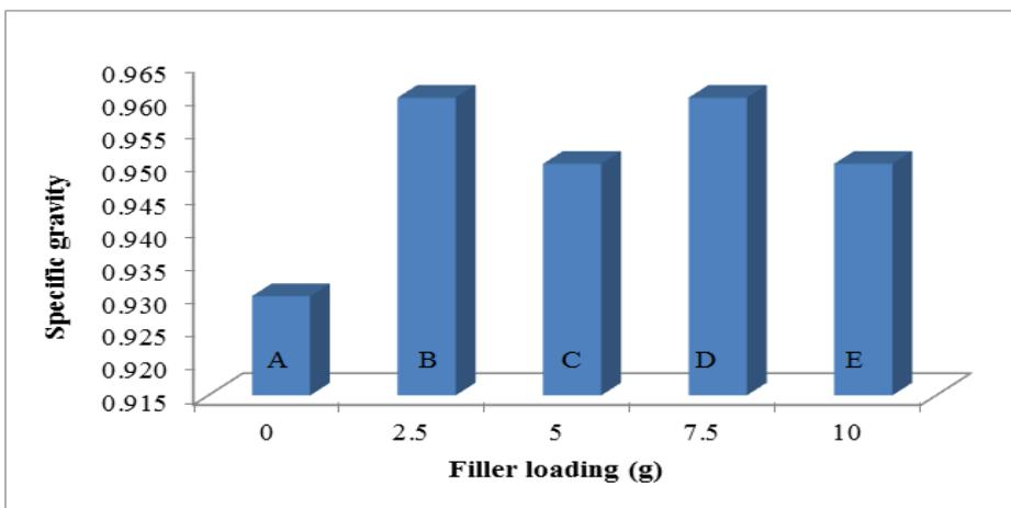
**Figure 5:** Specific gravity of natural rubber latex chitosan composites (A-E)
