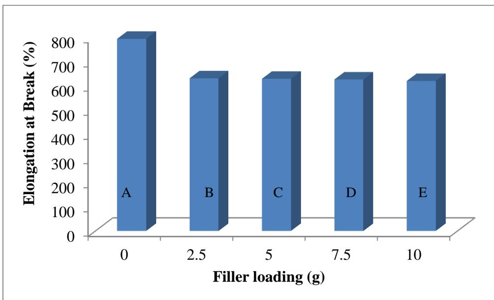
**Figure 7:** Elongation at break of natural rubber latex chitosan composites (A-E)
