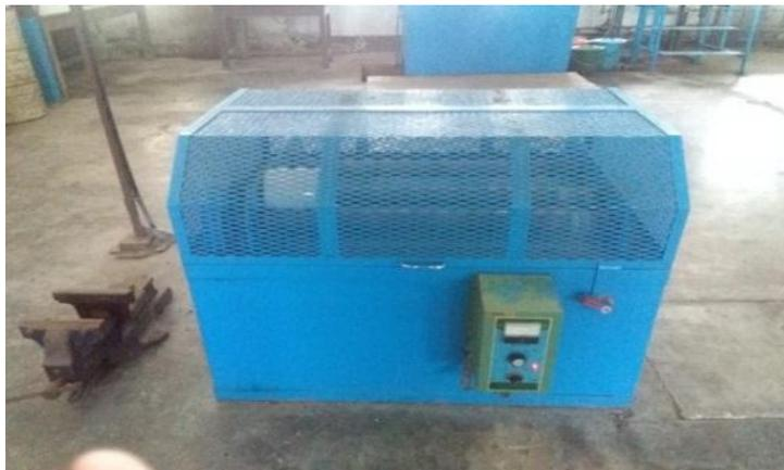
**Figure 3:** Ball mill machine
