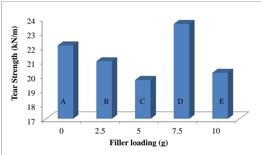
**Figure 9:** Tear strength of natural rubber latex chitosan composites (A-E)
