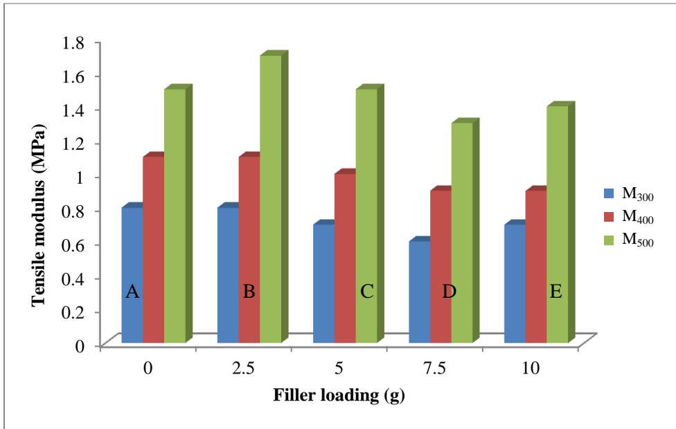
**Figure 8:** Tensile modulus of natural rubber latex chitosan composites (A-E)
