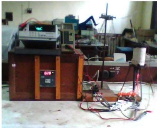
**Figure 3.** Photograph of the experimental setup of temperature dependent electrical resistance measurement
