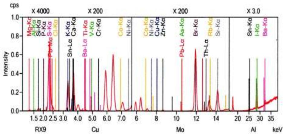
Figure 4 Spectrum of elemental concentration in seaweed from Waegali by NEXCG Spectrometer
