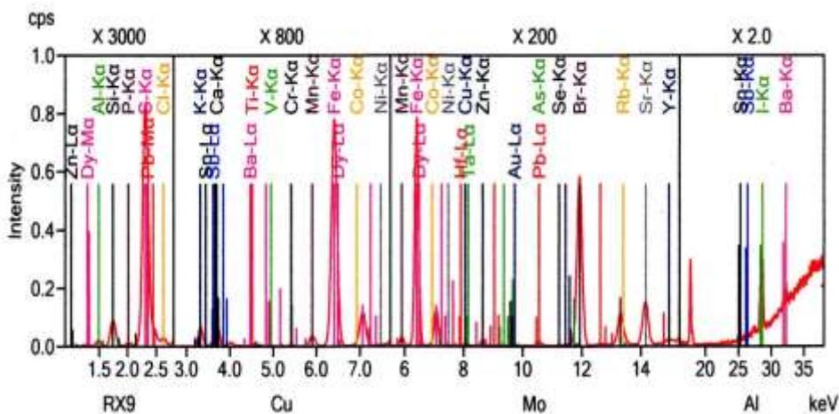
Figure 6 Spectrum of elemental concentration in seaweed from Kyaikkhami by NEXCG Spectrometer
