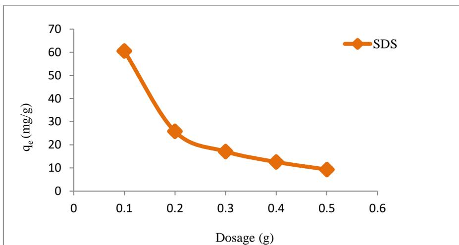
**Figure 3** Effect of dosage of HASSP-7 on the adsorption of SDS
