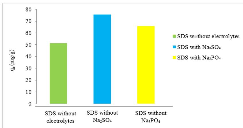
**Figure 4** Adsorption of SDS with and without electrolytes on HASSP-7
