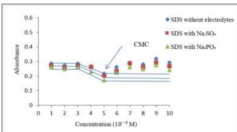
**Figure 1** Critical micelle concentration (CMC) of SDS with and without electrolytes
