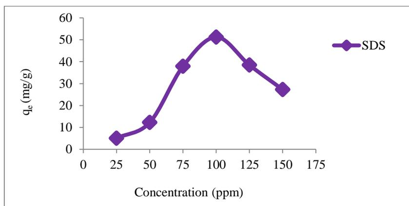
**Figure 2** Effect of initial concentration of SDS on the adsorption of SDS by HASSP-7
