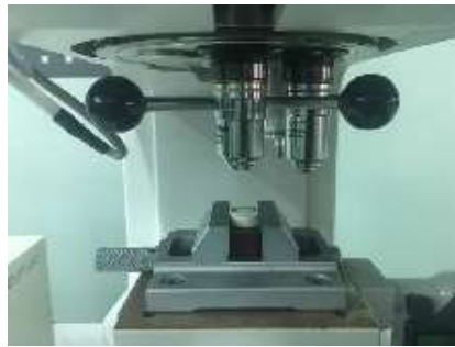
Figure 11 .Hardness measuring of F.S.HAp.-Glass Powder-GIC Composite with Mistutoyo Micro-hardness testing machine
