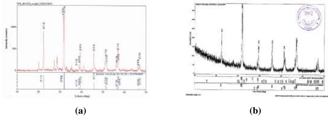
**Figure 1.** XRD patterns of (a) BiFeO<sub>3</sub> (b) Ag-BiFeO<sub>3</sub> powder
