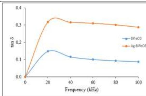
**Figure 5.** Comparison of dielectric loss tangent of BiFeO<sub>3</sub> and Ag-BiFeO<sub>3</sub> samples
