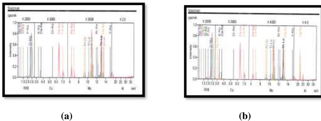
**Figure 2.** EDXRF spectra of (a) BiFeO<sub>3</sub>, (b) Ag-BiFeO<sub>3</sub> powder
