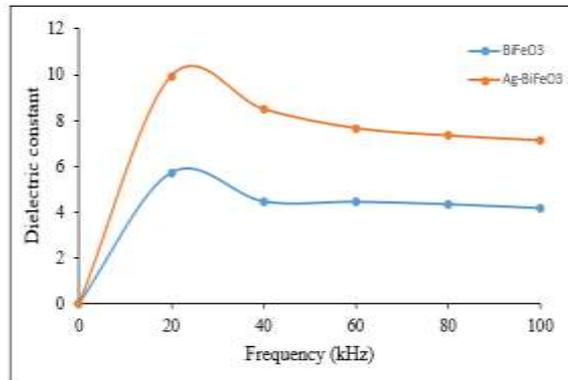
**Figure 4.** Comparison of dielectric constant of BiFeO<sub>3</sub> and Ag-BiFeO<sub>3</sub> samples
