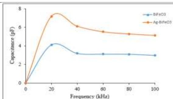
**Figure 6.** Comparison of capacitance of  $\text{BiFeO}_3$  and  $\text{Ag-BiFeO}_3$  samples
