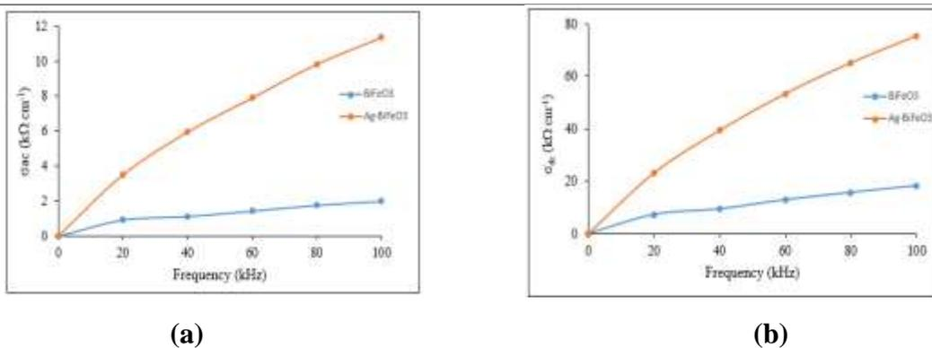
**Figure 3.** Comparison of (a) AC conductivity and (b) DC conductivity of BiFeO<sub>3</sub> and Ag-BiFeO<sub>3</sub> samples
