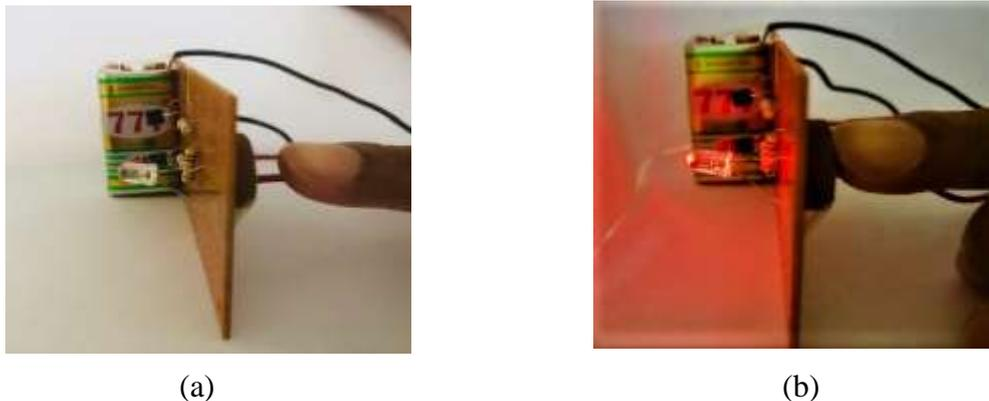
**Figure 8.** (a) Before touch onto the Ag-BiFeO<sub>3</sub> electrode (b) After touch onto the Ag-BiFeO<sub>3</sub> electrode
