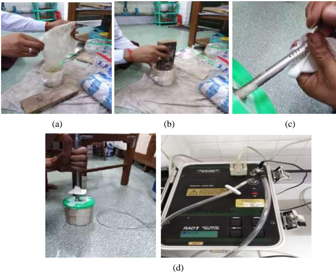
**Figure 4** (a), (b), (c) and (d) The photographs of the laboratory preparations for the detection of soil samples.
