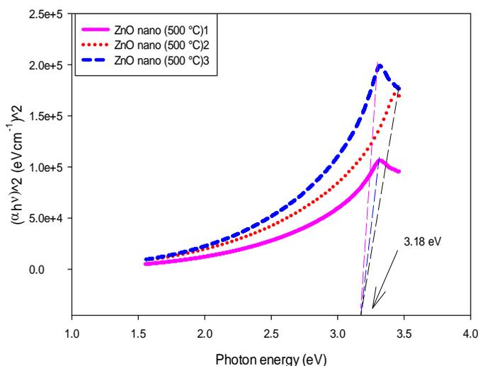
**Figure 5** Optical band gap of ZnO nanoparticles with different powder concentration at 500°C
