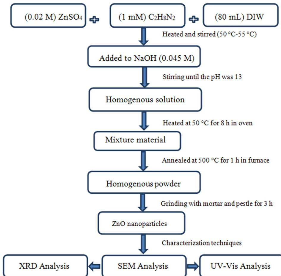
**Figure 1** Synthesis and characterization flow chart of ZnO nanoparticles at 500 °C
