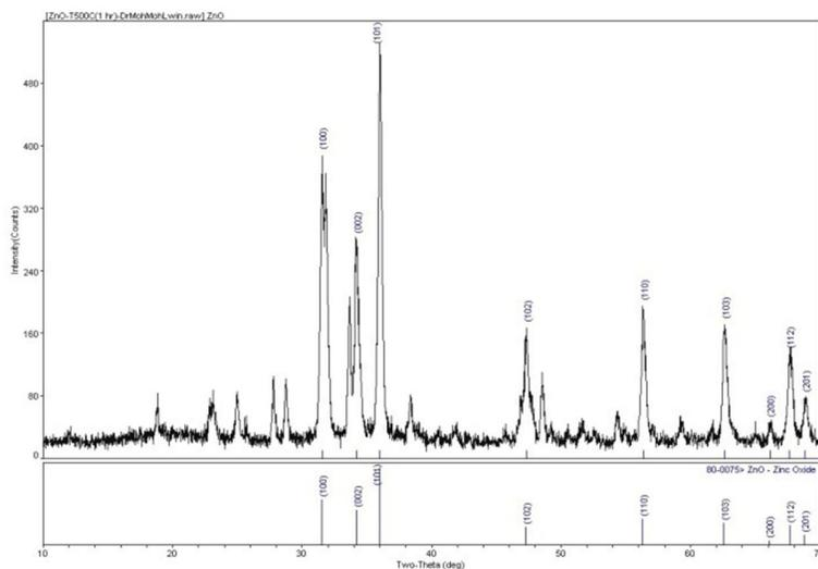
**Figure 2** XRD pattern of ZnO nanoparticles at 500 °C
