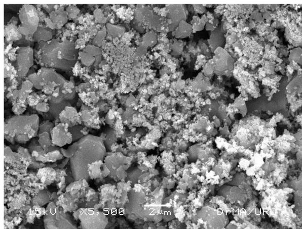
**Figure 3** SEM image of ZnO nanoparticles at 500 °C
