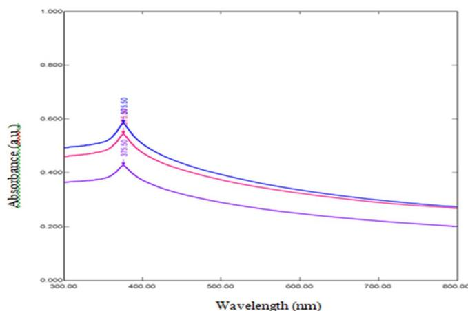
**Figure 4** Absorption spectrum of ZnO nanoparticles with different powder concentration at 500 °C
