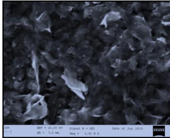
**Figure 5** SEM image of spin coated  $Ti_3C_2$  thin film on Si Substrate.
