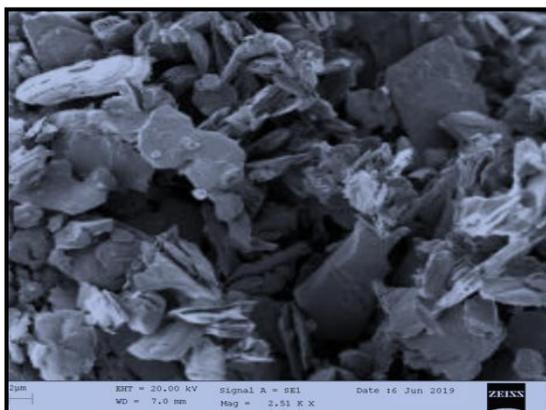
**Figure 3** The SEM micrograph of obtained MAX phase  $Ti_3AlC_2$  powders.
