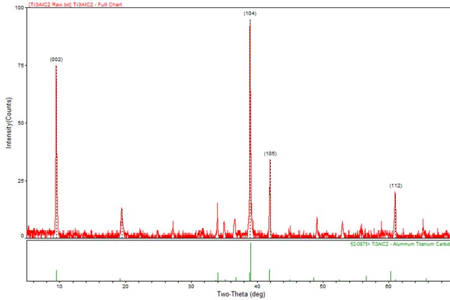
Figure 1 XRD profile of obtained MAX phase  $Ti_3AlC_2$  powder.
