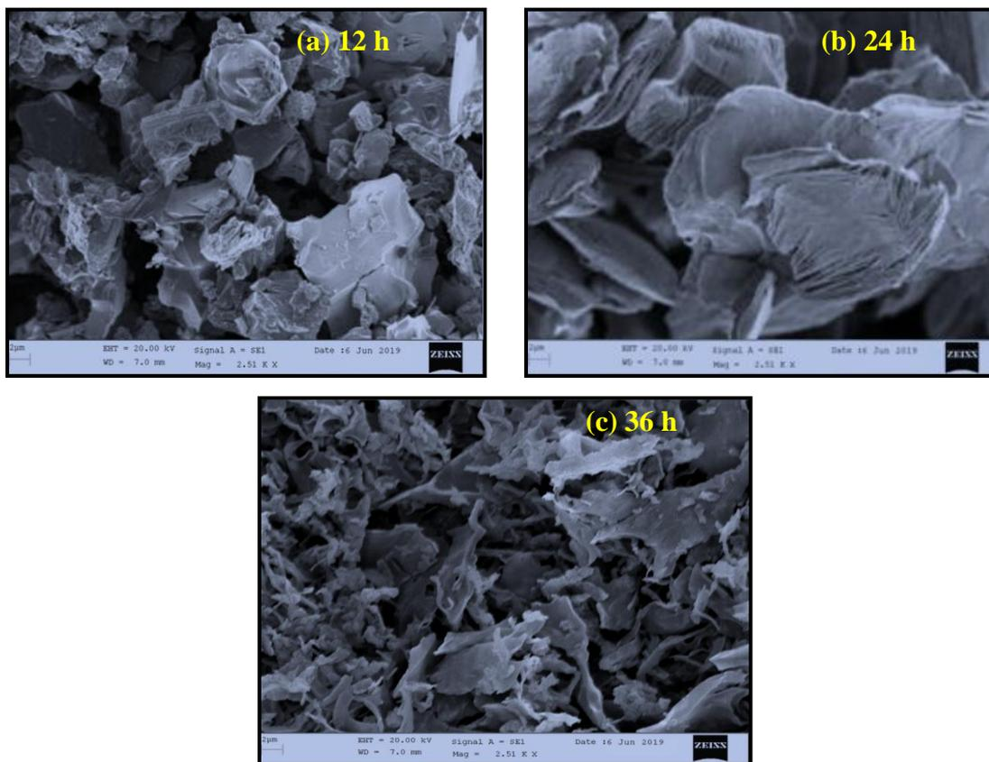
**Figure 4** SEM images of exfoliated  $Ti_3C_2$  for different etching time (a) 12 h (b) 24h and (c) 36 h.
