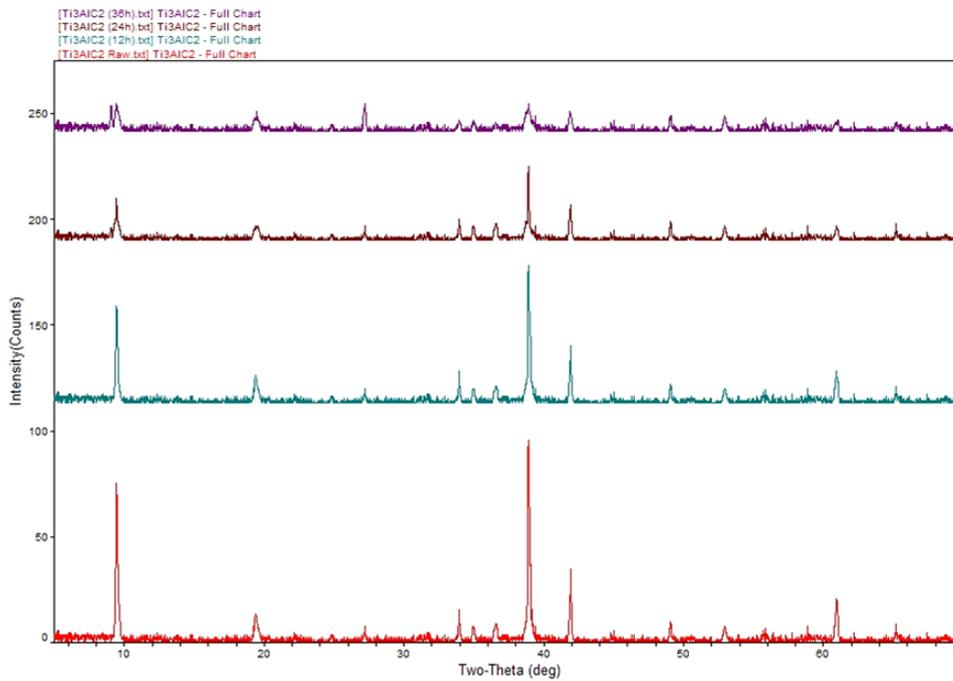
Figure 2 XRD patterns for HCl exfoliated powder for 12 h, 24 h and 36 h.
