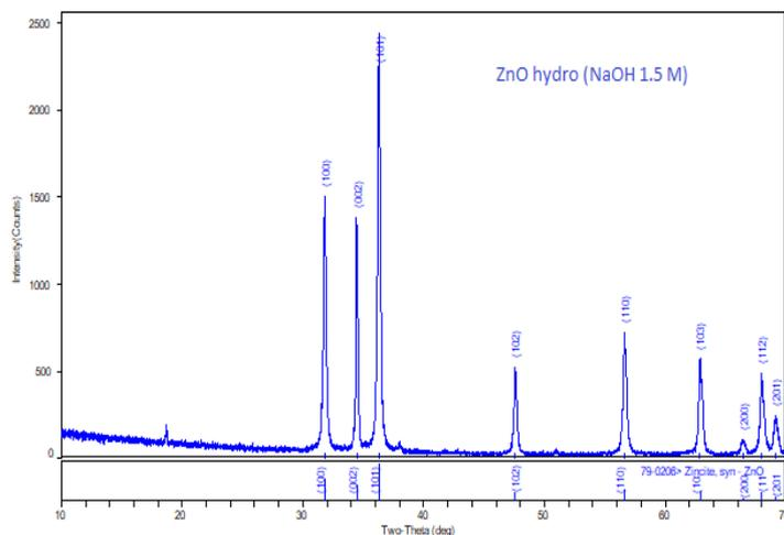
**Figure 2** XRD patterns of ZnO Nps by hydrothermal synthesis with (1.5 M NaOH)
