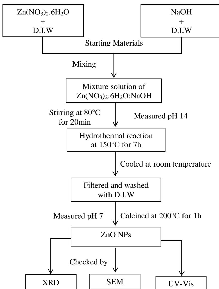
**Figure 1** The block diagram for the preparation ZnO nanoparticles
