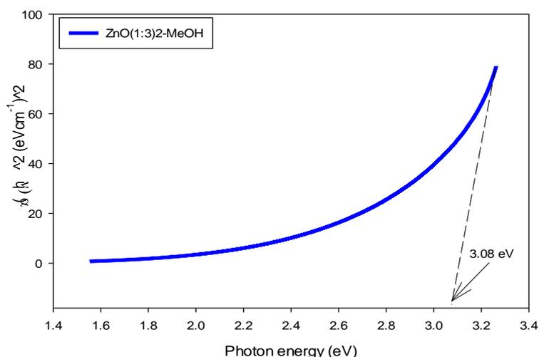
**Figure 6 (b)** Tauc's plot of ZnO NPs with (1.5 M NaOH)
