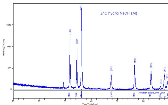
**Figure 1** XRD patterns of ZnO NPs by hydrothermal synthesis with (1M NaOH)
