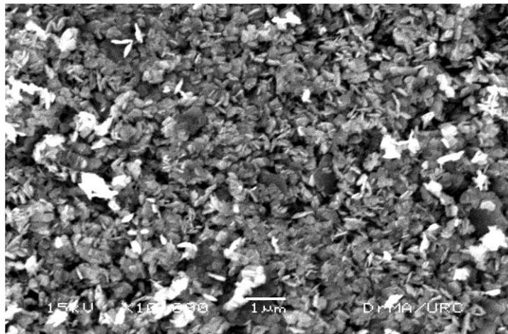
**Figure 4** SEM micrograph of ZnO crystals with bath molarity of NaOH(1.5 M)
