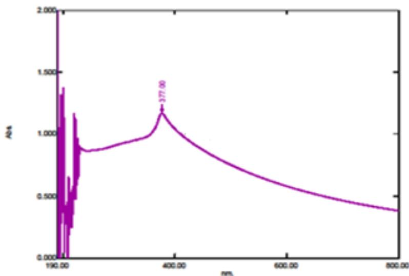
**Figure 6 (a)** Absorption spectrum of ZnO NPs with (1.5 M NaOH )
