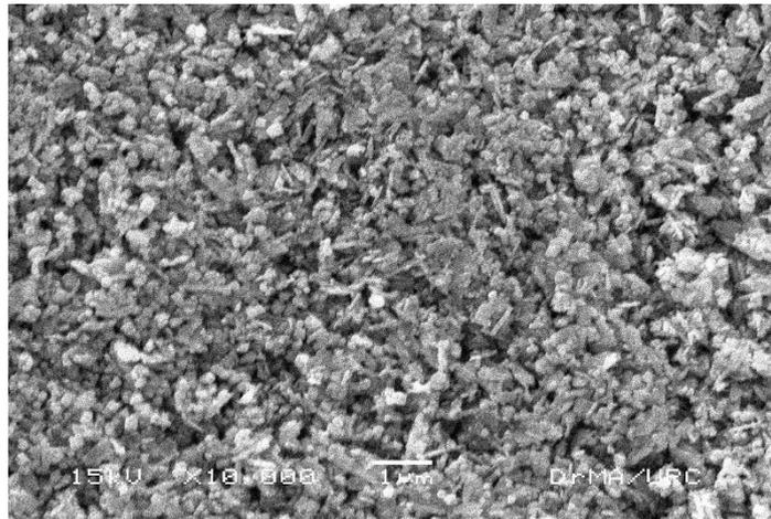
**Figure 3** SEM micrograph of ZnO crystals with bath molarity of NaOH ( 1 M)
