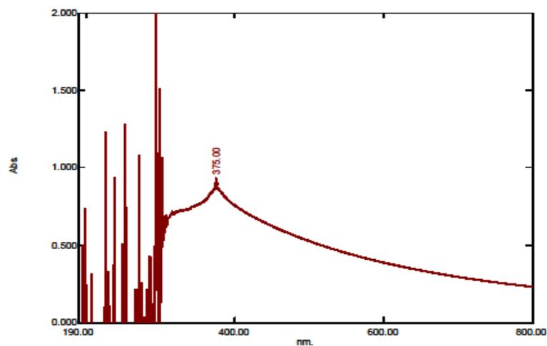
**Figure 5(a)** Absorption spectrum of ZnO NPs with (1 M NaOH )
