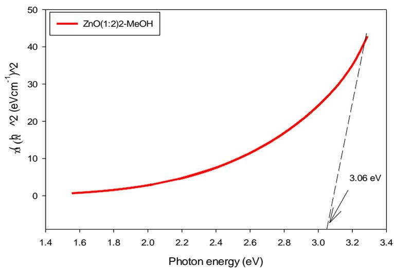
**Figure 5(b)** Tauc's plot of ZnO NPs with (1 M NaOH )
