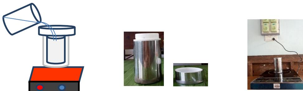
**Figure 2** Schematic diagram of home made Teflon-lined stainless steel vessel
