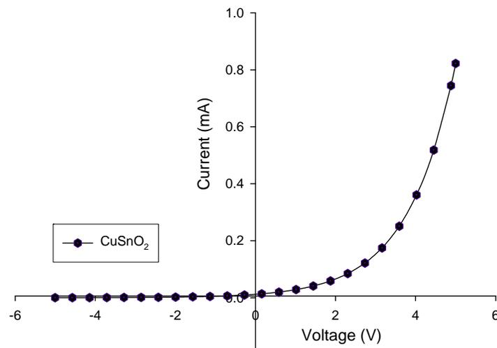
Figure 3 (b) I-V characteristics of (Cu doped SnO<sub>2</sub>)
