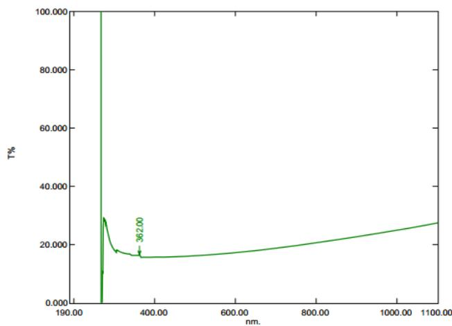
Figure 1 (b) Transmittance (T%) spectra for Cu doped SnO<sub>2</sub> thin film on glass
