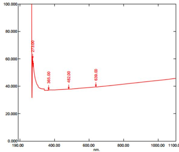
Figure 1 (a) Transmittance (T%) spectra for undoped SnO<sub>2</sub> thin film on glass
