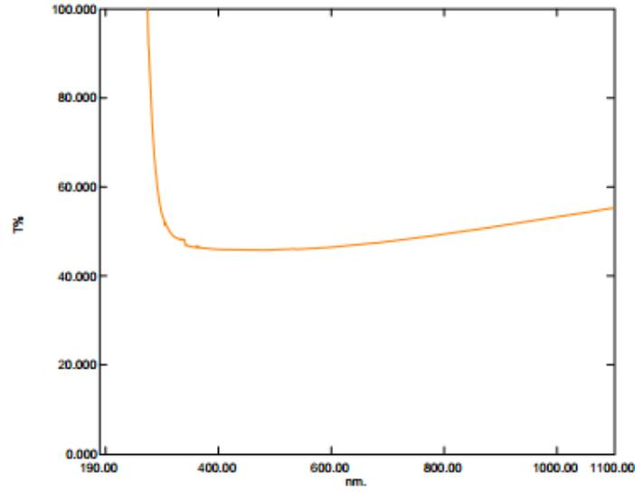
**Figure 1 (c)** Transmittance (T%) spectra for Al doped SnO<sub>2</sub> thin film on glass
