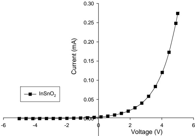
Figure 3 (d) I-V characteristics of (In doped SnO<sub>2</sub>)
