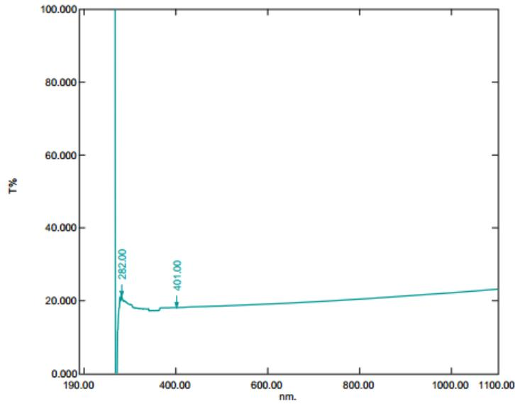
**Figure 1 (d)** Transmittance (T%) spectra for In doped SnO<sub>2</sub> thin film on glass
