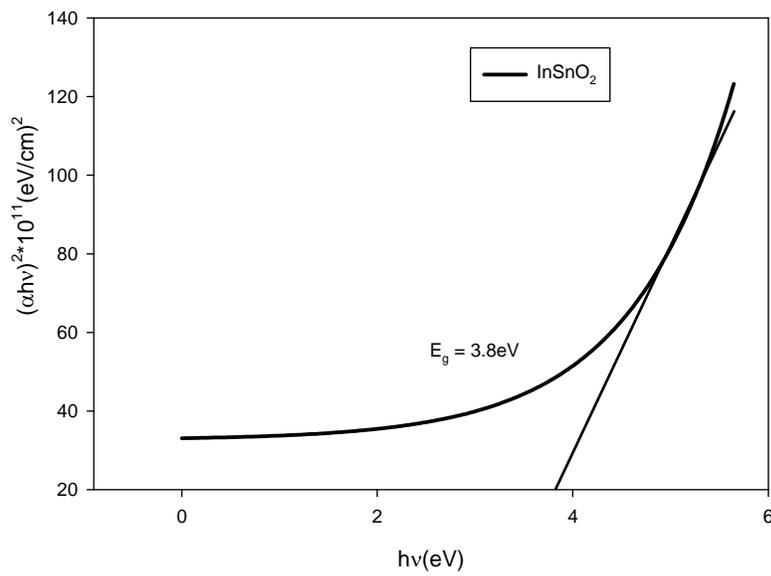
**Figure 2 (d)** Plot of  $(\alpha h\nu)^2$  versus  $h\nu$  ( In doped SnO<sub>2</sub>)
