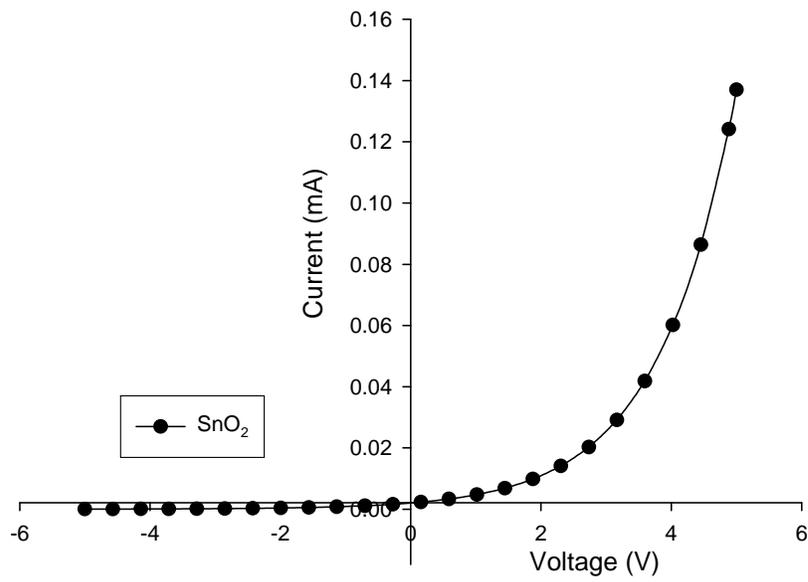
Figure 3 (a) I-V characteristics of (Undoped SnO<sub>2</sub>)
