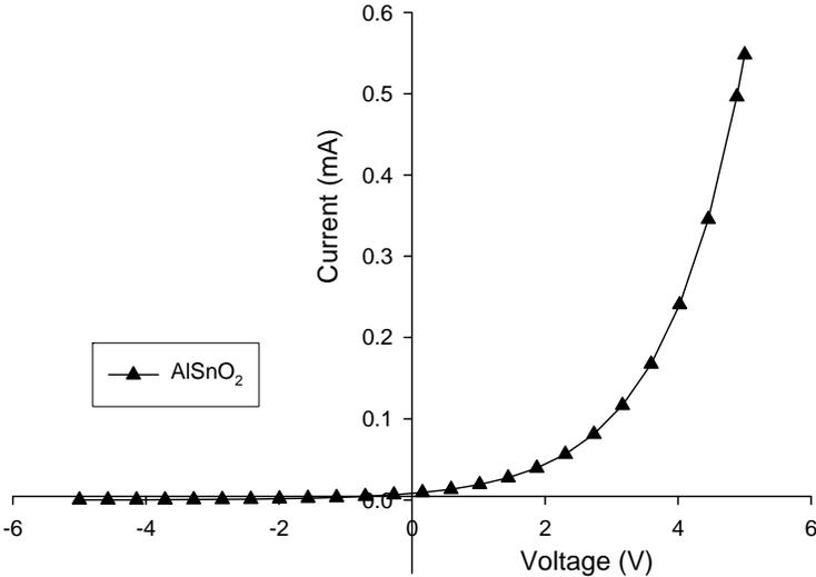
Figure 3 (c) I-V characteristics of (Al doped SnO<sub>2</sub>)
