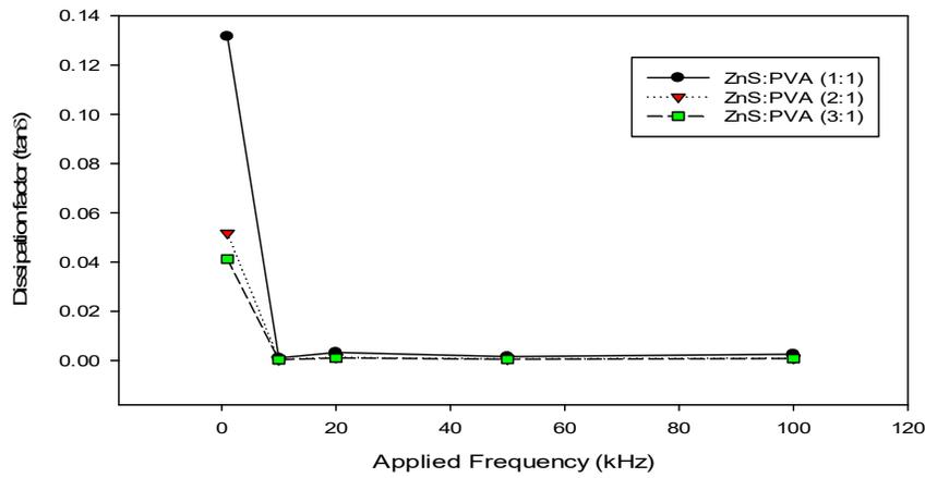
**Figure. 4(b)** Dissipation factor and frequency characteristic of ZnS /PVA films
