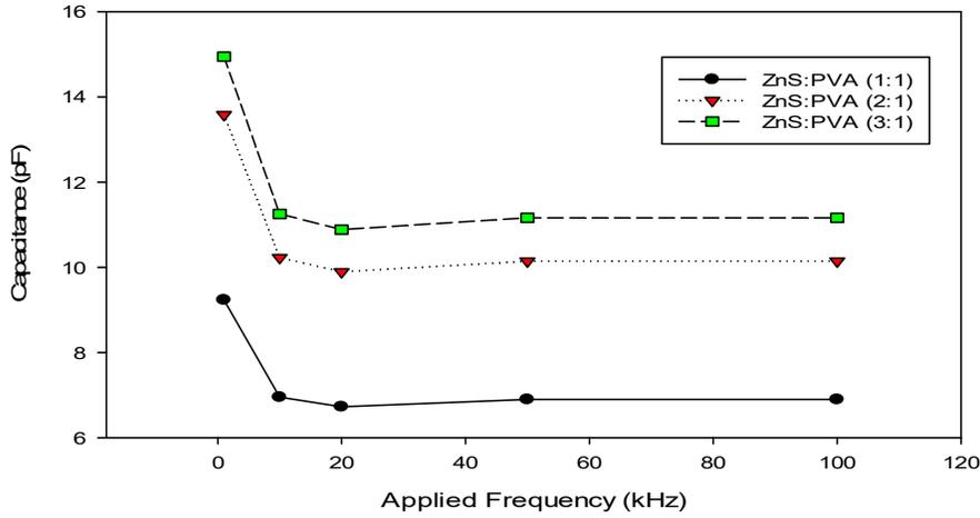
**Figure. 4(a)** Capacitance and frequency characteristic of ZnS/PVA films
