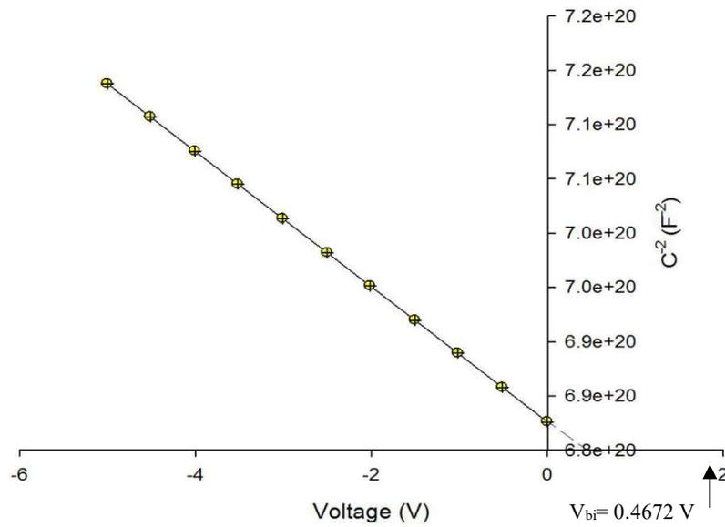
Figure.5 (c)  $1/C^2$ -V characteristic of fabricated film with ZnS:PVA (3:1)
