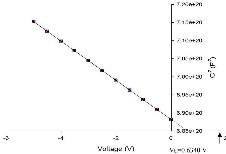
**Figure.5 (a)**  $1/C^2$ - $V$  characteristic of fabricated film with ZnS:PVA (1:1)
