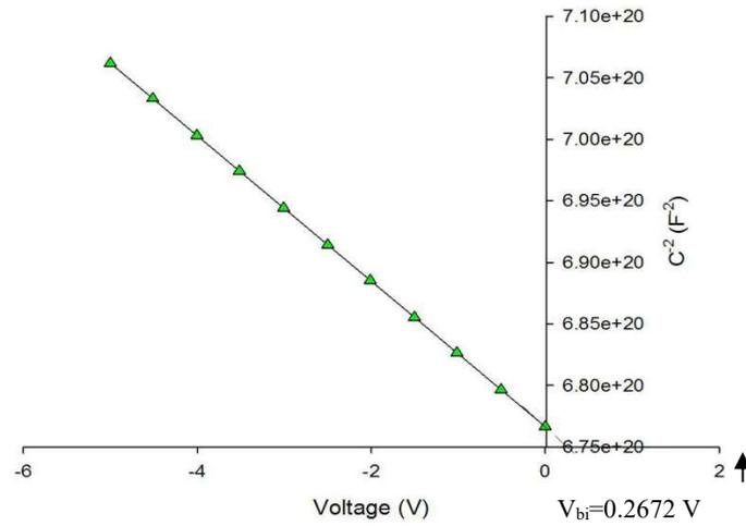
Figure. 5 (b)  $1/C^2$ -V characteristic of fabricated film with ZnS:PVA (2:1)
