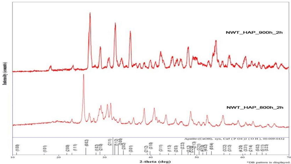
**Figure 5:** XRD diffractograms of HAP compare with calcination temperature (800°C) and sintering temperature (900°C)
