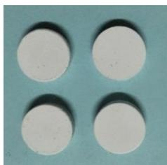
**Figure 1:** HAP/ $\beta$ -TCP pellets before sintering temperature
