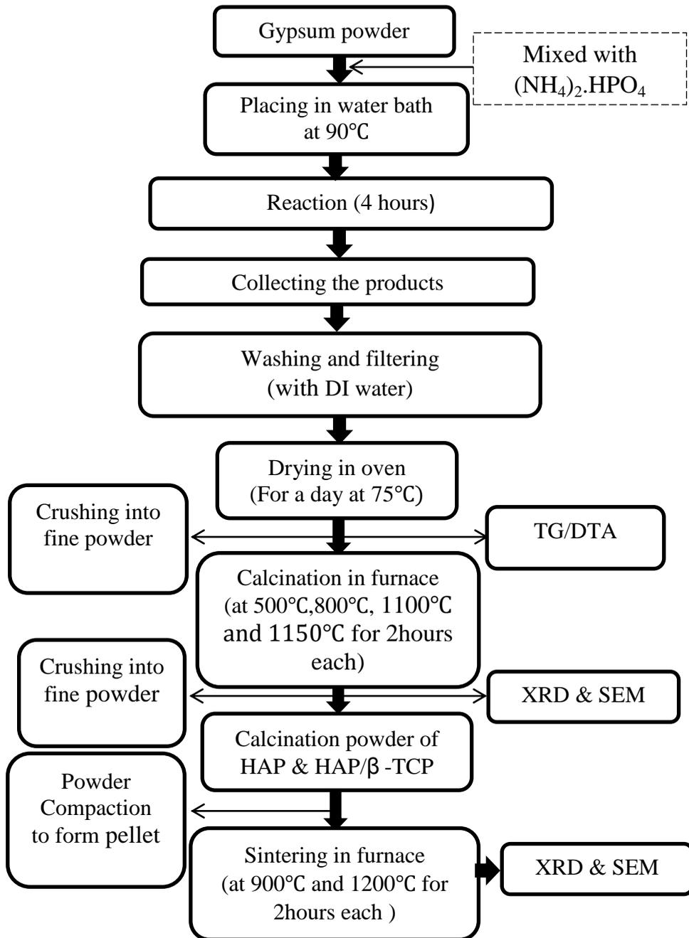
**Figure 2:** Flowchart of HAP and HAP/β-TCP sample
