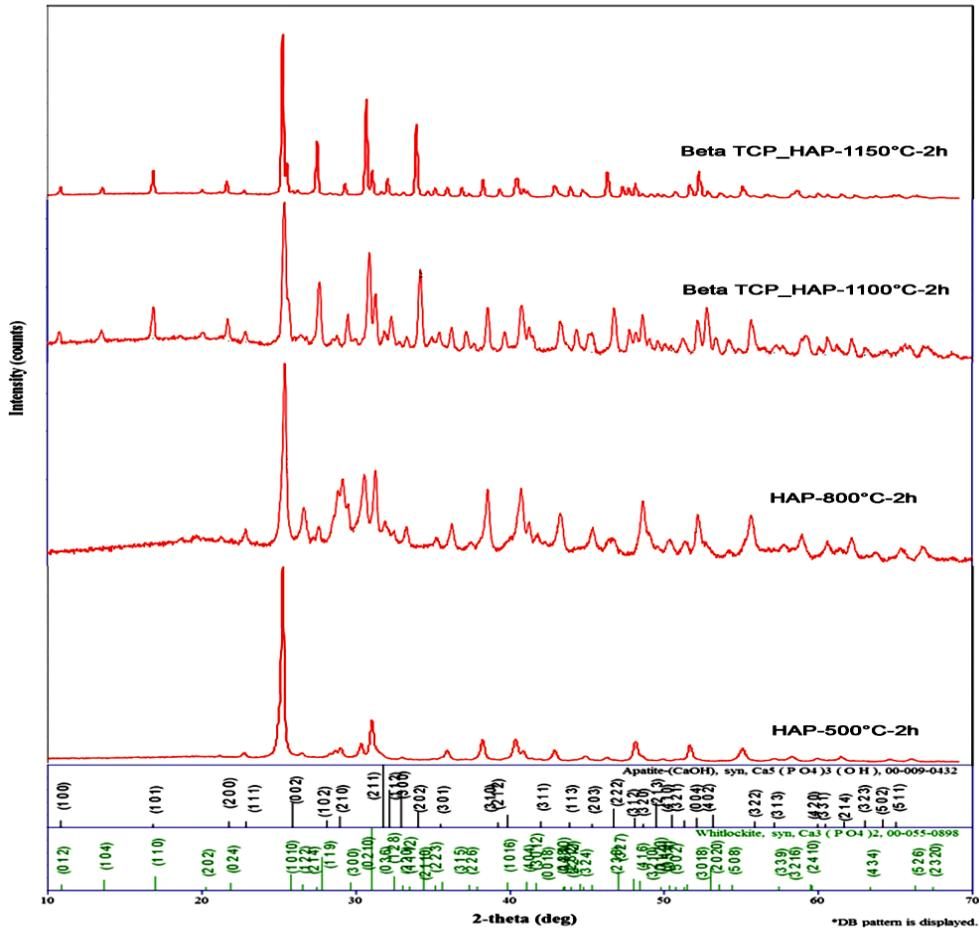
Figure 4: XRD diffractograms of HAP and  $\beta$ -TCP powder for different temperatures
