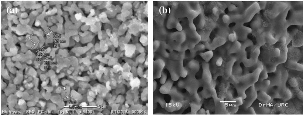
**Figure 8:** The SEM micrographs of the HAP pellet at (a) 900°C and that of HAP/ $\beta$ -TCP pellet at (b) 1200°C for 2 hours
