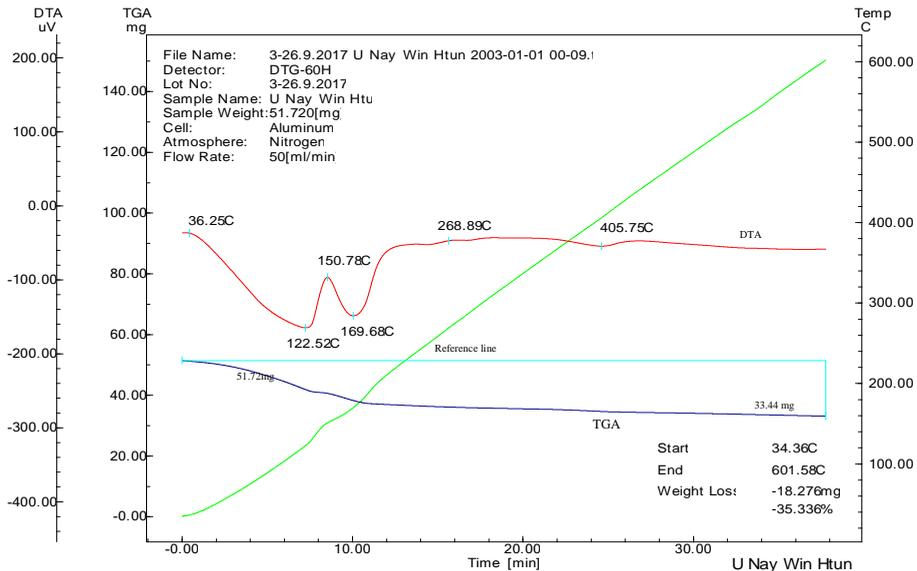
**Figure 3:** A plot of TG/DTA for the thermal behavior of the co-precipitated gypsum and di-ammonium hydrogen phosphate compound
