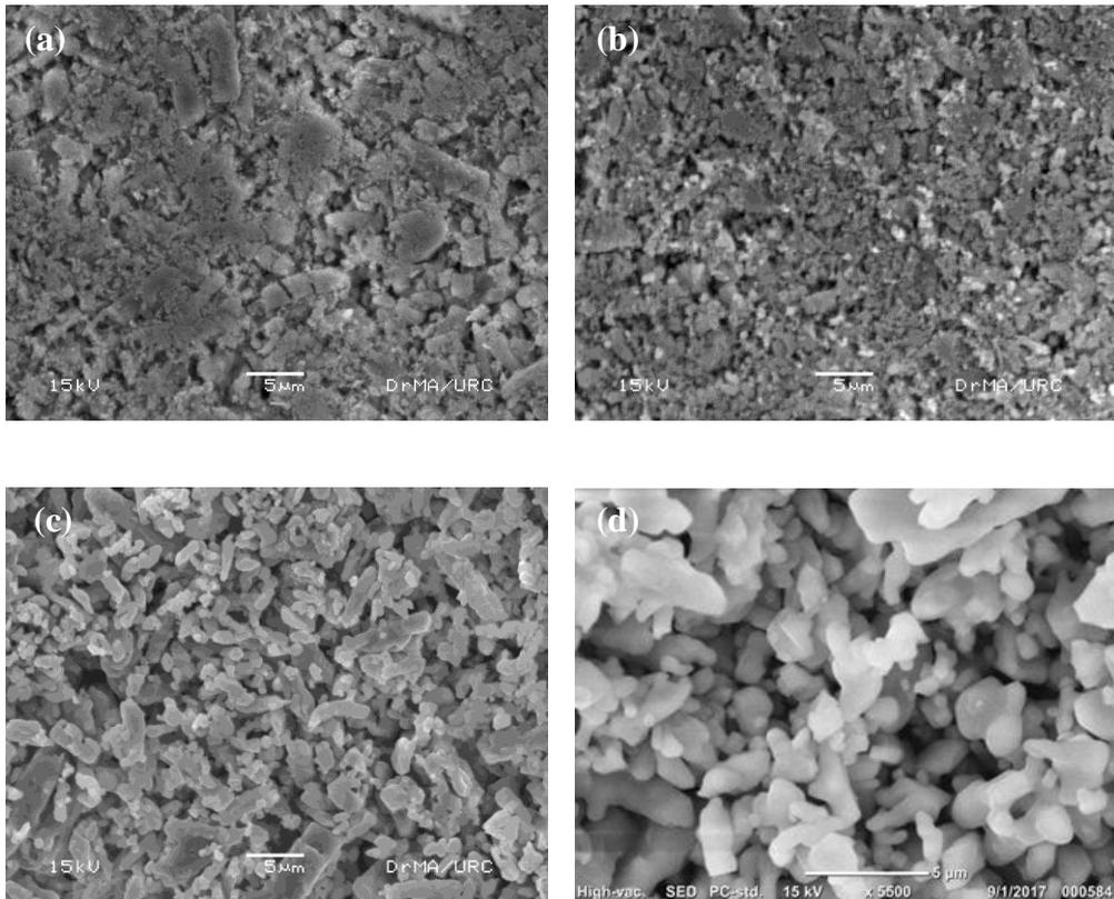
**Figure 7:** The SEM micrographs of the HAP powder at (a) 500°C, (b) 800°C and that of HAP/ $\beta$ -TCP powder at (c) 1100°C, (d) 1150°C for 2hours
