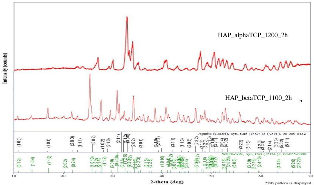
**Figure 6:** XRD diffractograms of HAP,  $\beta$ -TCP and  $\alpha$ -TCP compare with calcination temperature (1100°C) and sintering temperature (1200°C)
