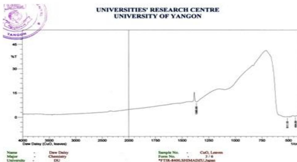
**Figure 11** FT IR spectrum of the prepared CuO NPs by using leaves extract
