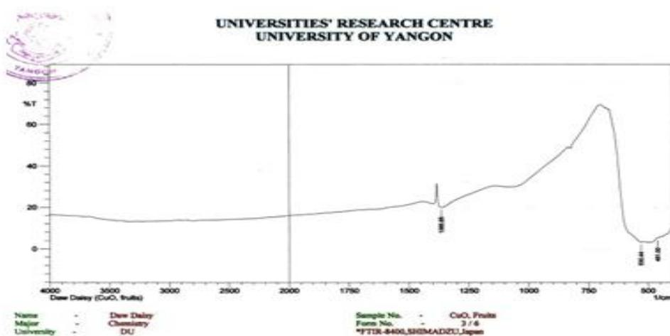
**Figure 12** FT IR spectrum of the prepared CuO NPs by using fruits extract
