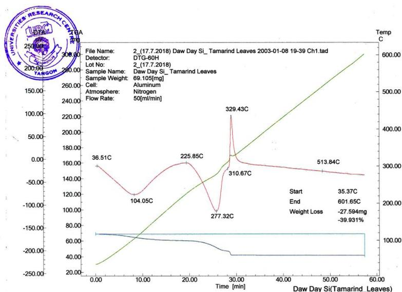
**Figure 9** TG-DTA thermogram of the prepared CuO NPs by using leaves extracts of *T. indica*
