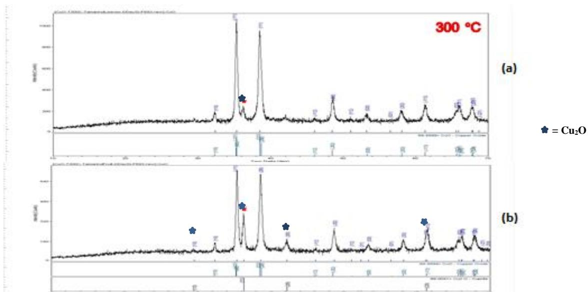
**Figure 2** X ray diffractogram of the prepared CuO NPs by using (a) leaves extract and (b) fruits extract of *T. indica* at 300 °C
