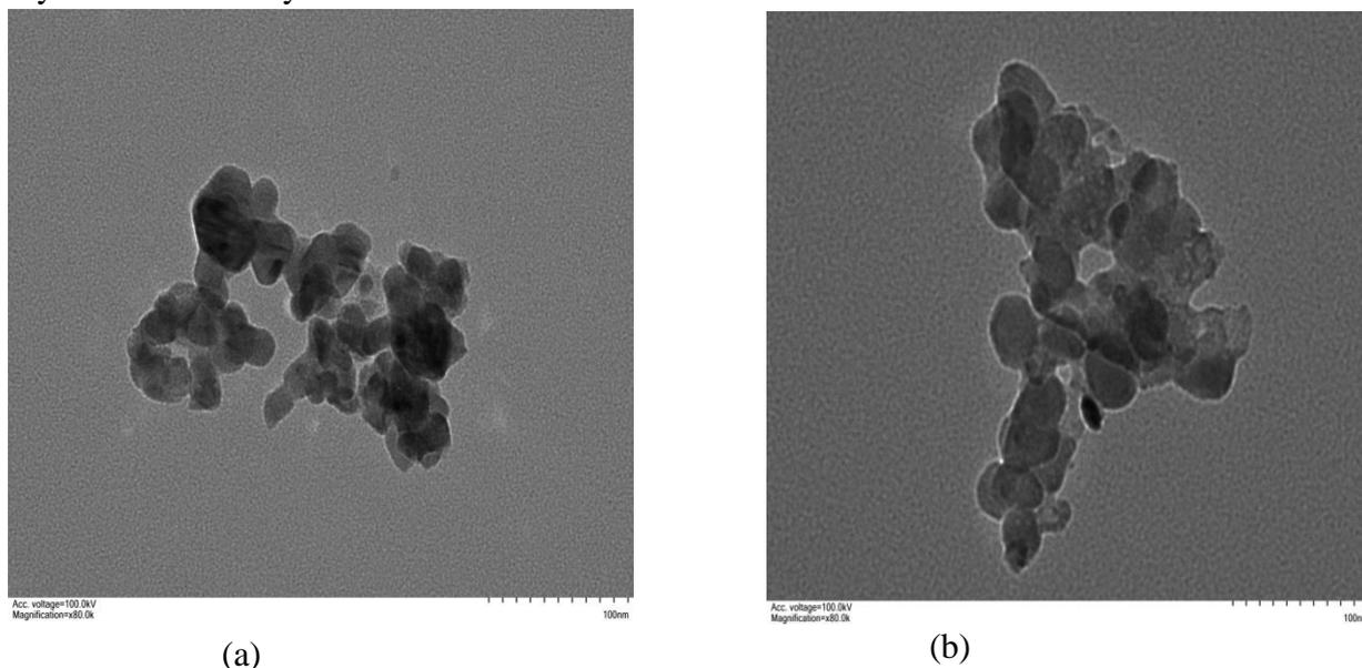
**Figure 8** TEM images of the prepared CuO NPs by using (a) leaves extract and (b) fruits extract of *T. indica* (Magnification= $\times 80.0k$ )
