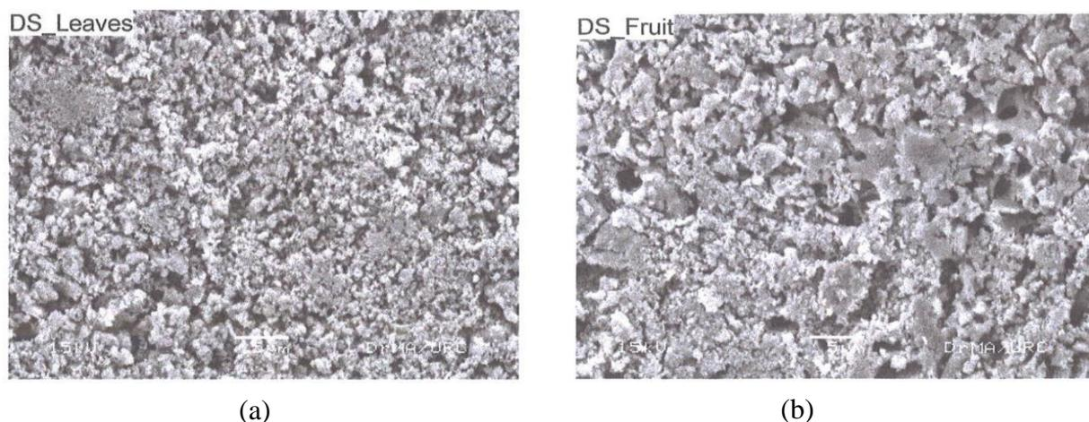
**Figure 7** SEM micrographs of the prepared CuO by using (a) leaves extract and (b) fruits extract of *T. indica*
