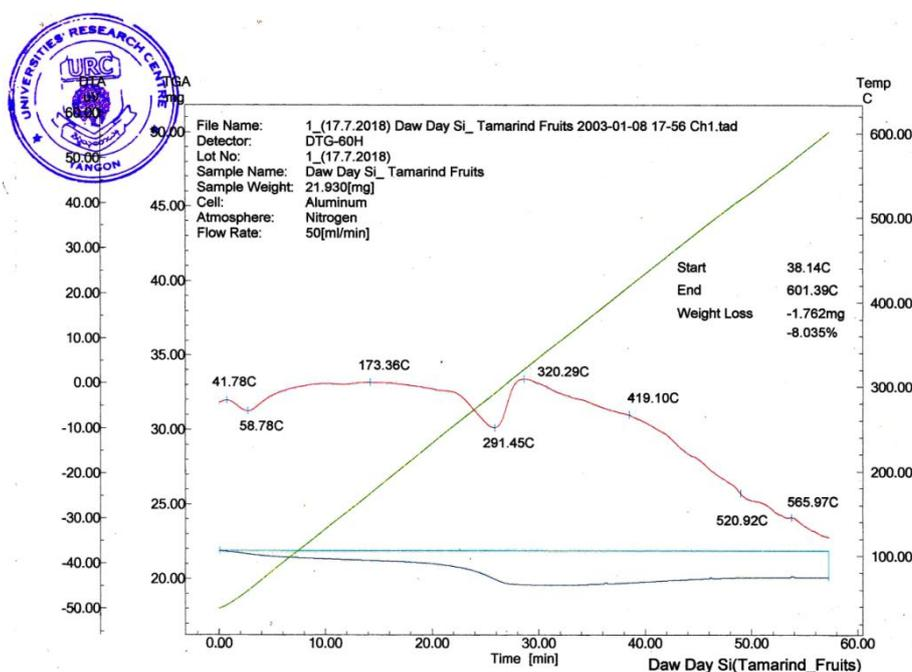
**Figure 10** TG-DTA thermogram of the prepared CuO NPs by using fruits extracts of *T. indica*
