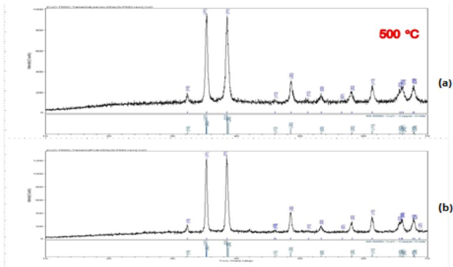
**Figure 4** X ray diffractogram of the prepared CuO NPs by using (a) leaves extract and (b) fruits extract of *T. indica* at 500 °C
