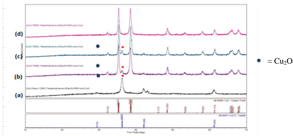
**Figure 5** Comparison of X ray diffractograms of the prepared CuO NPs by using leaves extract of *T. indica* at (a) 200 °C (b) 300 °C (c) 400 °C and (d) 500 °C
