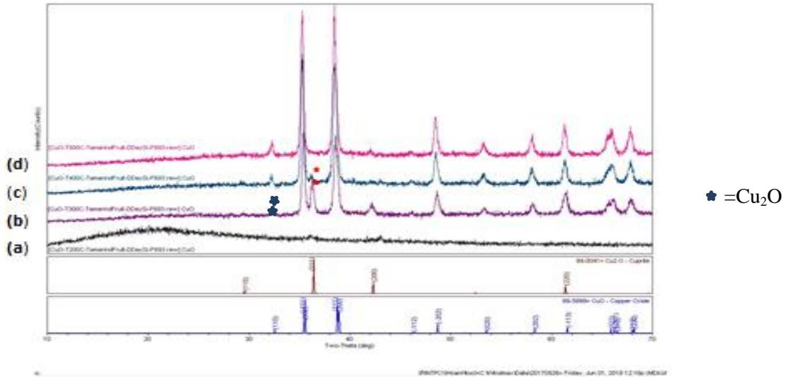
**Figure 6** Comparison of the X ray diffractograms of the prepared CuO NPs by using fruits extract of *T. indica* at (a) 200 °C (b) 300 °C (c) 400 °C and (d) 500 °C
