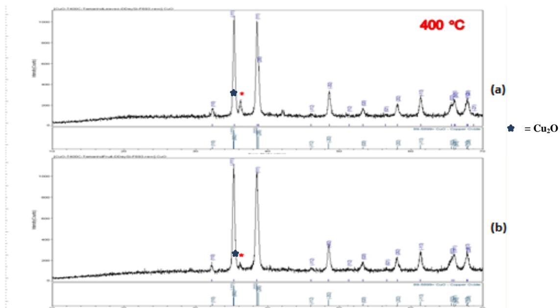
**Figure 3** X ray diffractogram of the prepared CuO NPs by using (a) leaves extract and (b) fruits extract of *T. indica* at 400 °C
