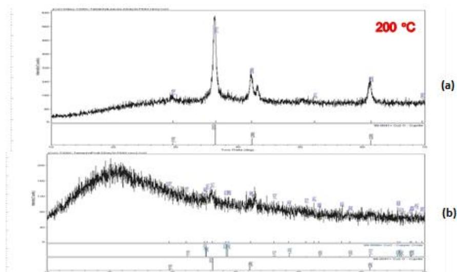
**Figure 1** X ray diffractogram of the prepared CuO NPs by using (a) leaves extract and (b)fruits extract of *T. indica* at 200 °C
