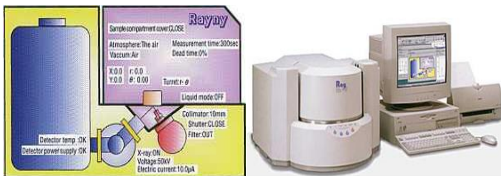
Figure 4: The functional diagram and photograph of EDX-720 spectrometer system
