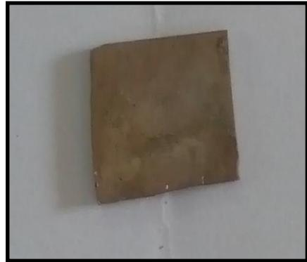
(b) Ag thin film annealed at 400° C
