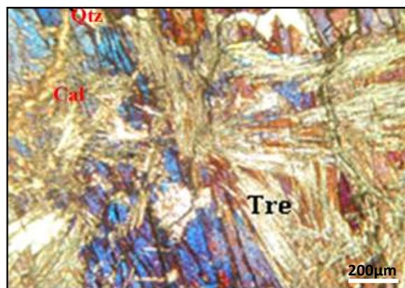
**Figure 7** Photomicrograph showing fibrous aggregate of tremolite in calc-silicate rock, (Under XN), Tre = Tremolite, Cal = Calcite and Qtz = Quartz
