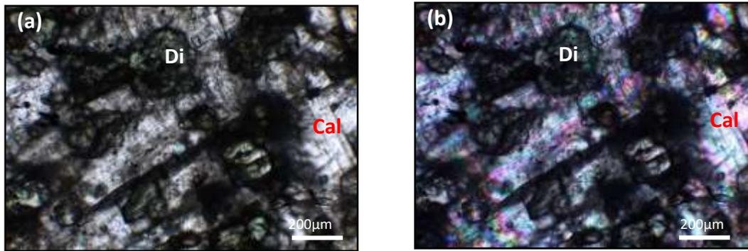
**Figure 5** Photomicrograph showing randomly oriented diopside grains (a) under PPL (b) under XN. Di=Diopside and Cal= Calcite
