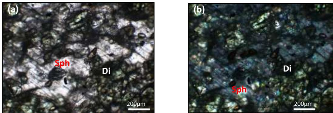
**Figure 6** Photomicrograph showing disseminated granules of sphene in calc-silicate rock (a) under PPL (b) under XN. Di=Diopside, Sph=Sphene
