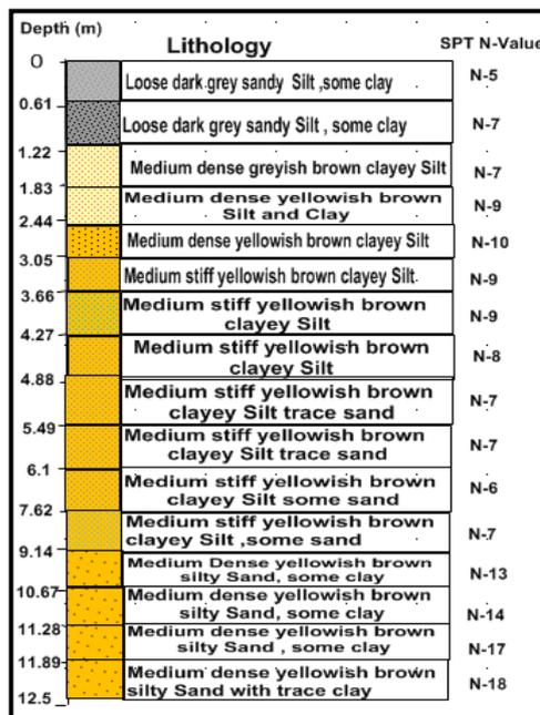
Figure 10 Subsurface soil profile of a site at 48<sup>th</sup> Street, Botahtaung Township
