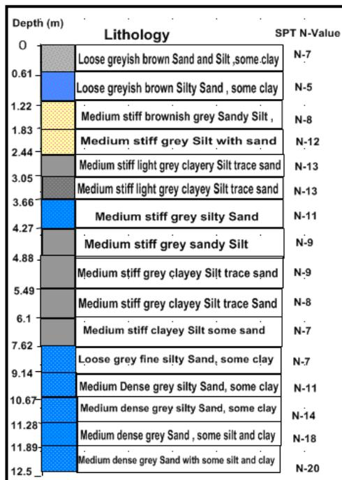
**Figure 7** Subsurface soil profile of a site at 21<sup>st</sup> Street, Latha Township
