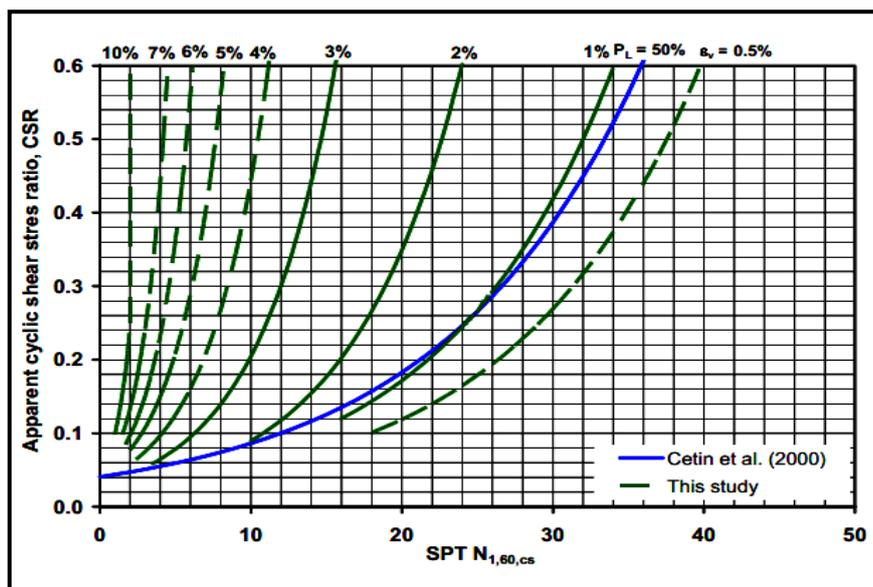
**Figure 6** Correlations between CSR, ( $N_1$ )<sub>60,cs</sub> and reconsolidation volumetric strain
