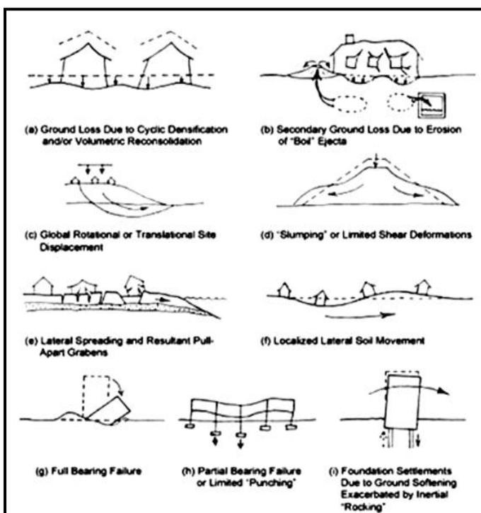
Figure 5 Illustration of liquefaction induced ground settlement mechanisms
