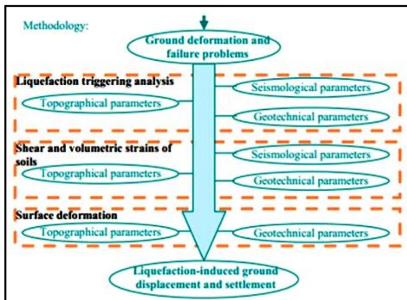
**Figure 2** Components of semi-empirical based method
