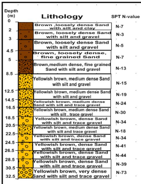
Figure 9 Subsurface soil profile of proposed Fly Over Project, Kyauktada Township
