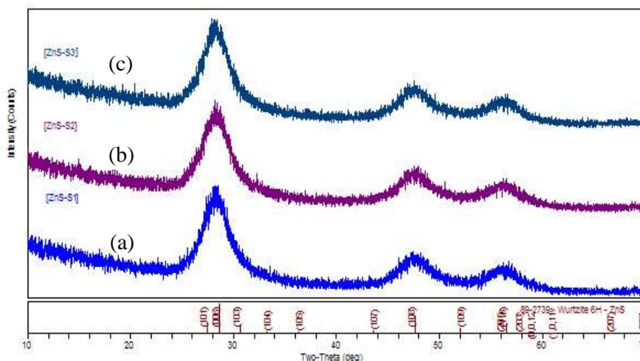
**Figure 1** XRD pattern of zinc sulphide nanoparticles using (a) 25 mL of honey (S1) (b) 50 mL of honey (S2) and (c) 75 mL honey (S3)
