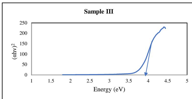
**Figure 8** Tauc plots for calculation of band gap energy values of zinc sulphide nanoparticles (S1, S2 and S3)
