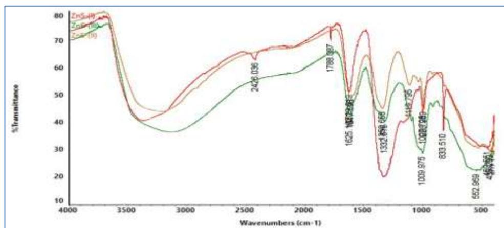
**Figure 6** FT IR spectra of zinc sulphide nanoparticles (S1, S2 and S3)
