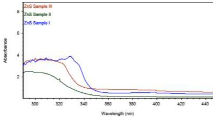
Figure 7 Absorption spectra of zinc sulphide nanoparticles (S1, S2 and S3)
