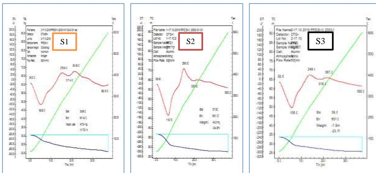
Figure 5 TG-DTA thermogram of zinc sulphide nanoparticles (S1, S2 and S3)
