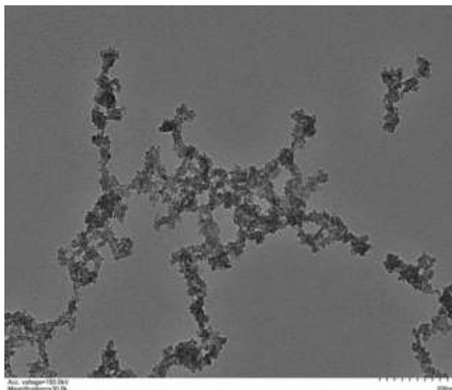
**Figure 2** TEM image of zinc sulphide nanoparticles using 25 mL of honey (S1)
