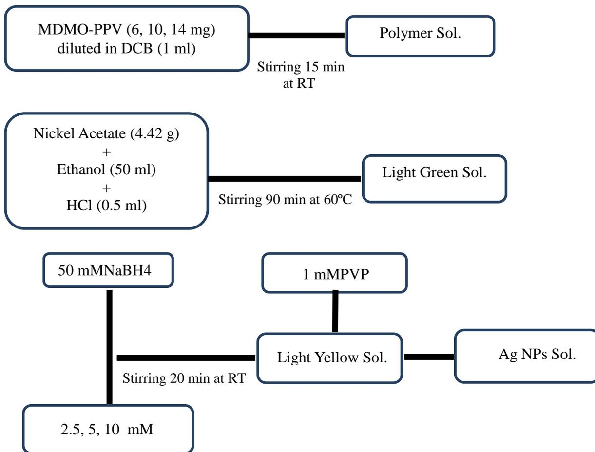
**Figure 1** Synthesis steps for polymer, NiO and Ag NPs solutions.
