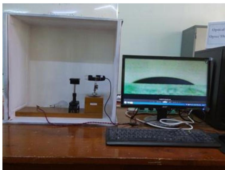
**Figure 2** The experimental setup for contact angle measurement.
