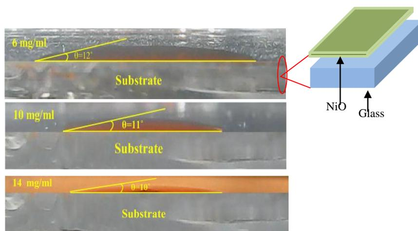
**Figure 3** Contact angles of polymer MDMO-PPV solution on NiO film at 700°C.
