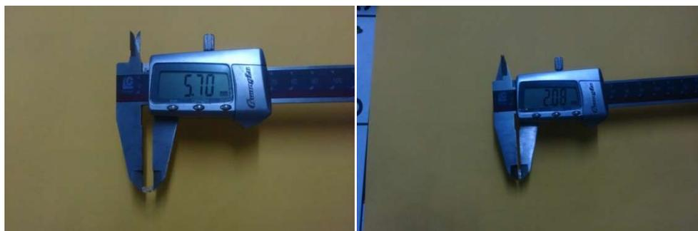
(q) Length of  $\text{Li}_2\text{SO}_4$  doped TGS
