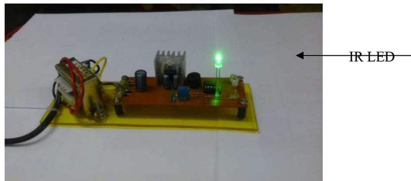
Figure 4.(c) IR driver circuit (Power ON) (Side-view / transmitted IR light source as an electrically ceramic light source)
