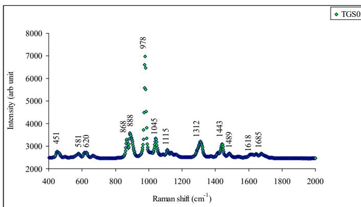
**Figure 5.(b)** Raman spectrum of  $K_2SO_4$  doped TGS crystal
