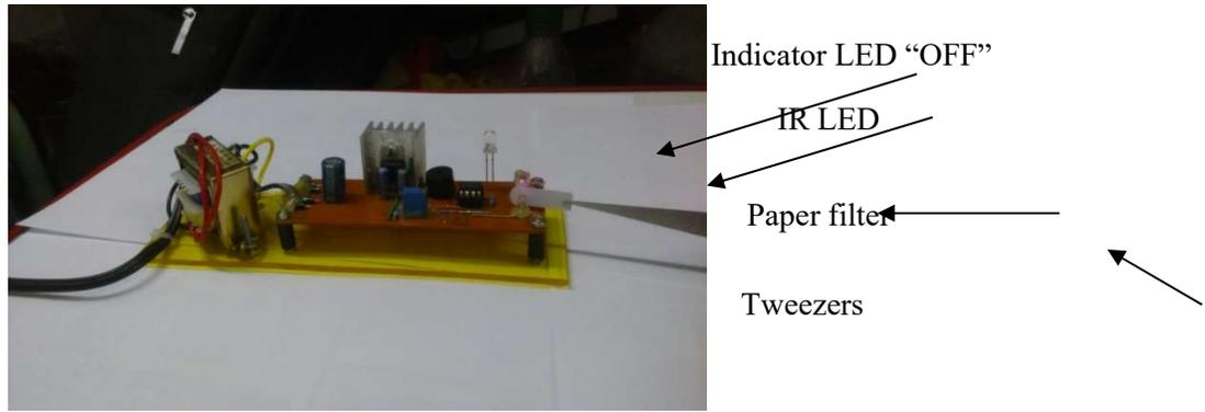
Figure 4(e). Testing of paper as an IR-filter
