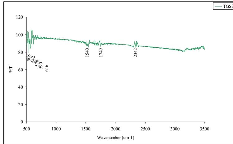
Figure 7.(c) FTIR transmission spectrum of (NH<sub>4</sub>)<sub>2</sub>SO<sub>4</sub> doped TGS crystal
