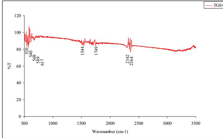
**Figure 7.(d)** FTIR transmission spectrum of Li<sub>2</sub>SO<sub>4</sub> doped TGS crystal
