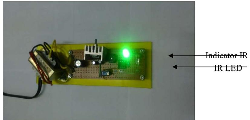
Figure 4.(b) IR driver circuit (Power ON) (Top-view)
