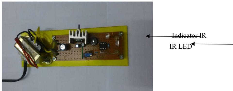
**Figure 4.(a)** IR driver circuit (Power OFF)
