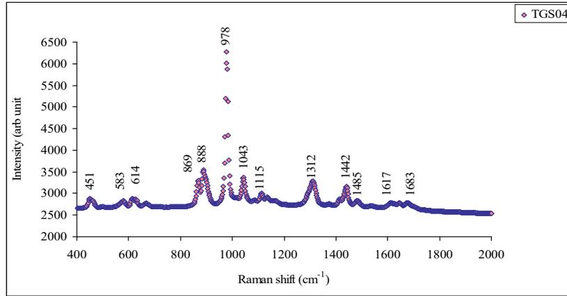
**Figure 5.(d)** Raman spectrum of  $\text{Li}_2\text{SO}_4$  doped TGS crystal
