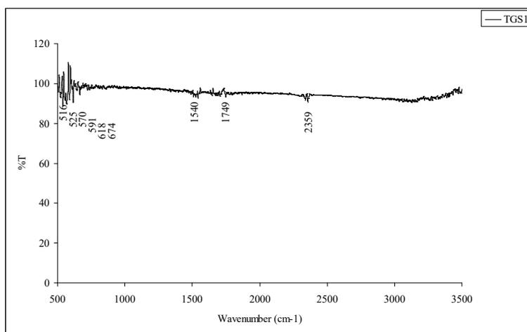
**Figure 7.(a)** FTIR transmission spectrum of undoped TGS crystal
