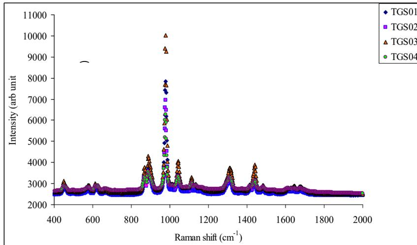
**Figure 6.** Raman spectra of undoped and  $\text{M}_2\text{SO}_4$  ( $\text{M} = \text{K}, \text{NH}_4, \text{Li}$ ) doped TGS crystals
