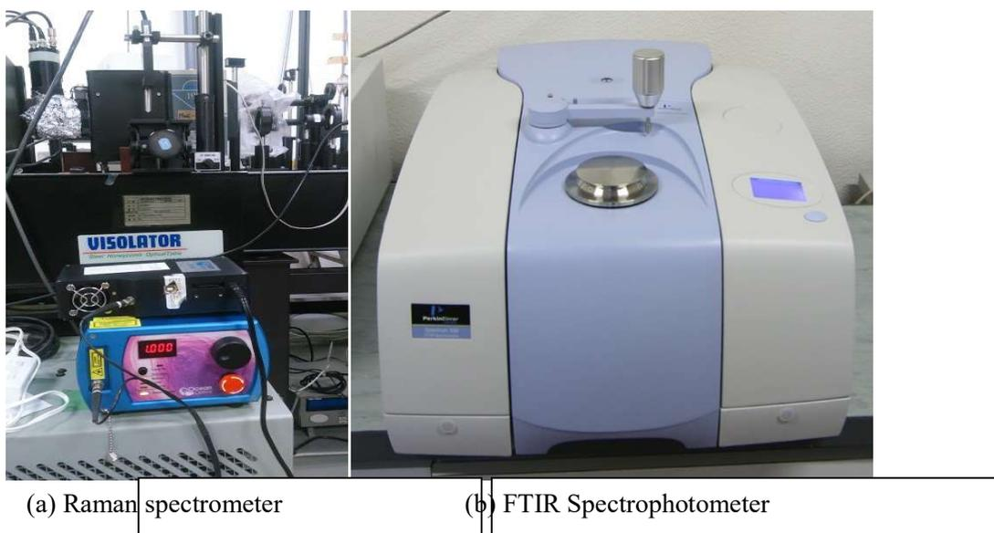
**Figure 3.** Photographs of (a) Ocean Optics QE65000 Visolator Laser Raman Spectrometer and (b) Perkin-Elmer Spectrum-100 FTIR Spectrophotometer
