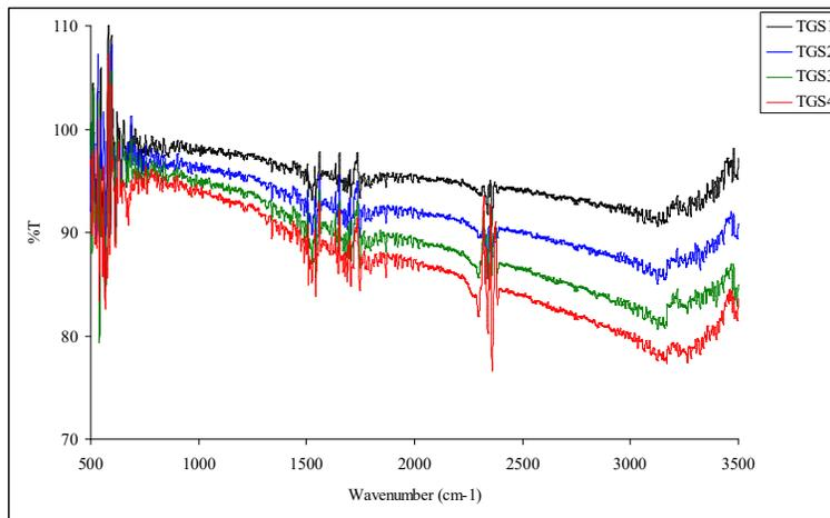
**Figure 8.** FTIR transmission spectra of undoped and M<sub>2</sub>SO<sub>4</sub> (where M = K, NH<sub>4</sub>, Li) doped TGS crystals
