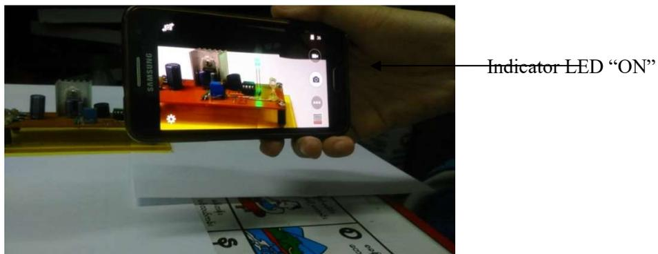
Figure 4(g). Testing of cell-phone camera with interaction of IR (indicator LED "ON")
