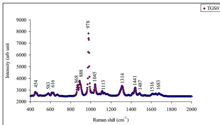
**Figure 5.(a)** Raman spectrum of undoped TGS crystal
