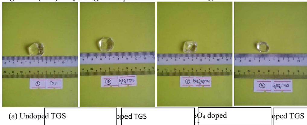
**Figure 1.** Photographs of (a) undoped TGS, (b)  $K_2SO_4$  doped TGS, (c)  $(NH_4)_2SO_4$  doped TGS and (d)  $Li_2SO_4$  doped TGS crystals
