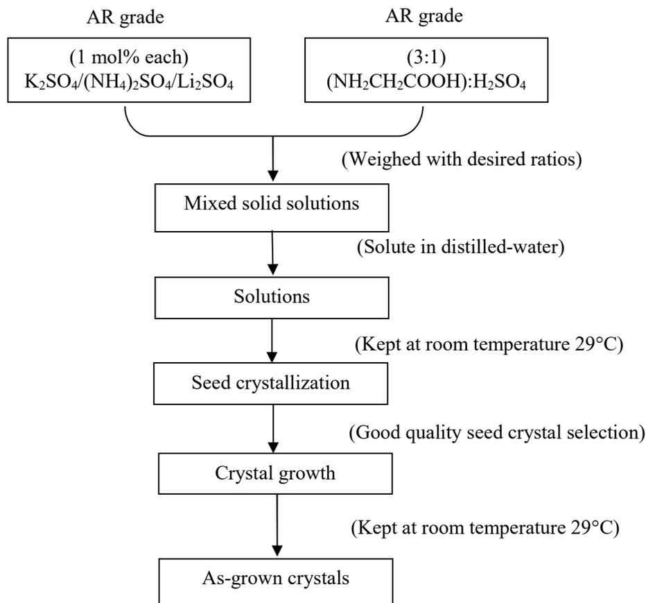
**Figure 2.** Flow diagram of the crystal growth process
