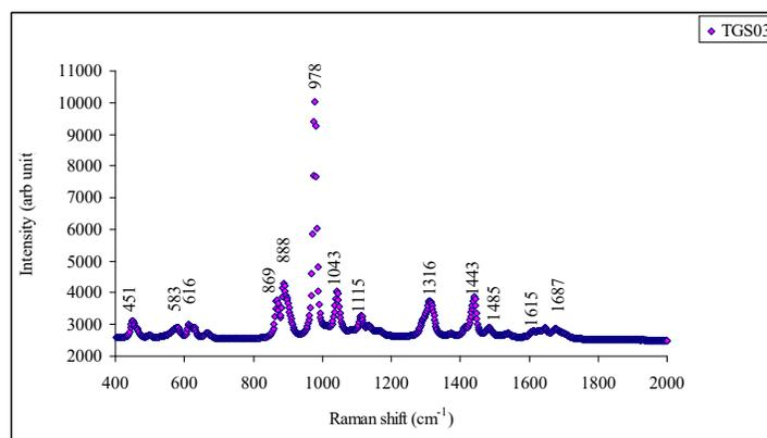
**Figure 5.(c)** Raman spectrum of  $(NH_4)_2SO_4$  doped TGS crystal
