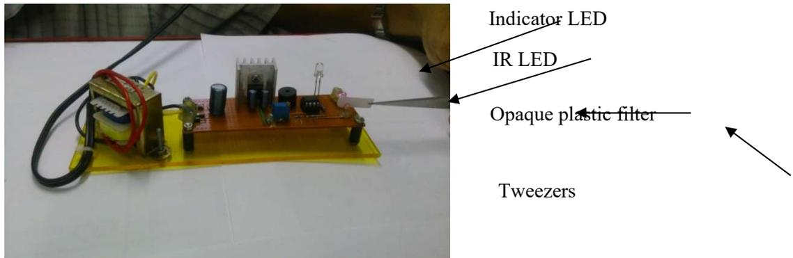
Figure 4.(f) Testing of thin opaque plastic as an IR-filter
