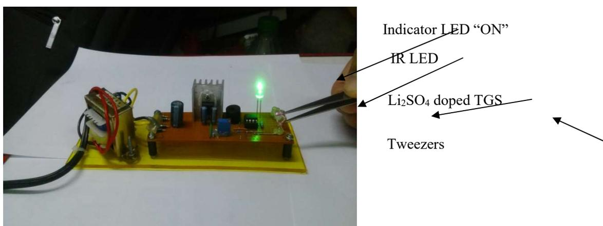
**Figure 4.(s)** Testing of IR windows material of  $\text{Li}_2\text{SO}_4$  doped TGS crystal
