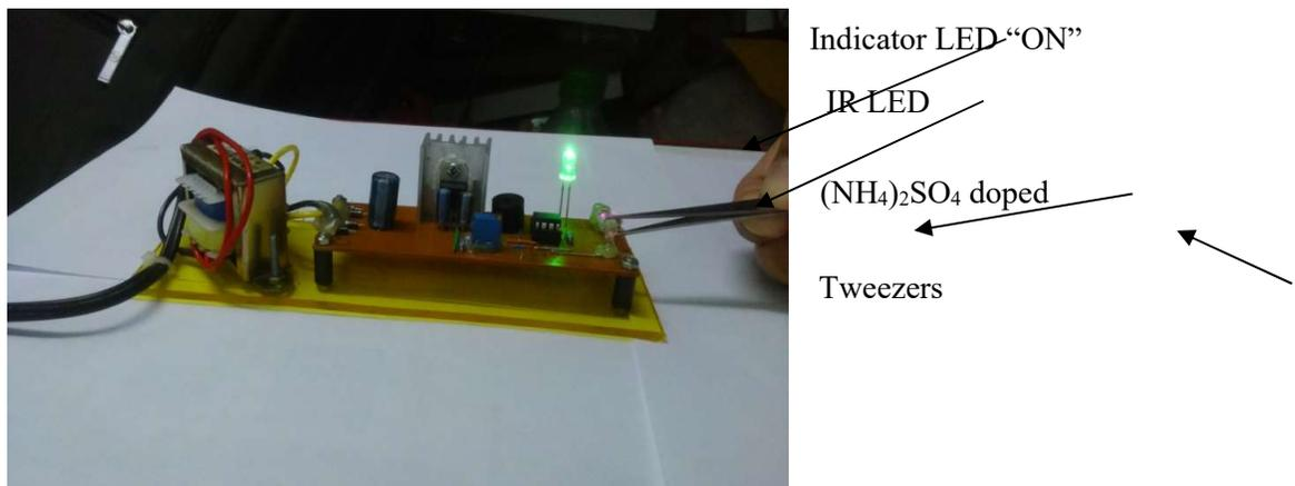
**Figure 4.(p)** Testing of IR windows material of  $(NH_4)_2SO_4$  doped TGS crystal
