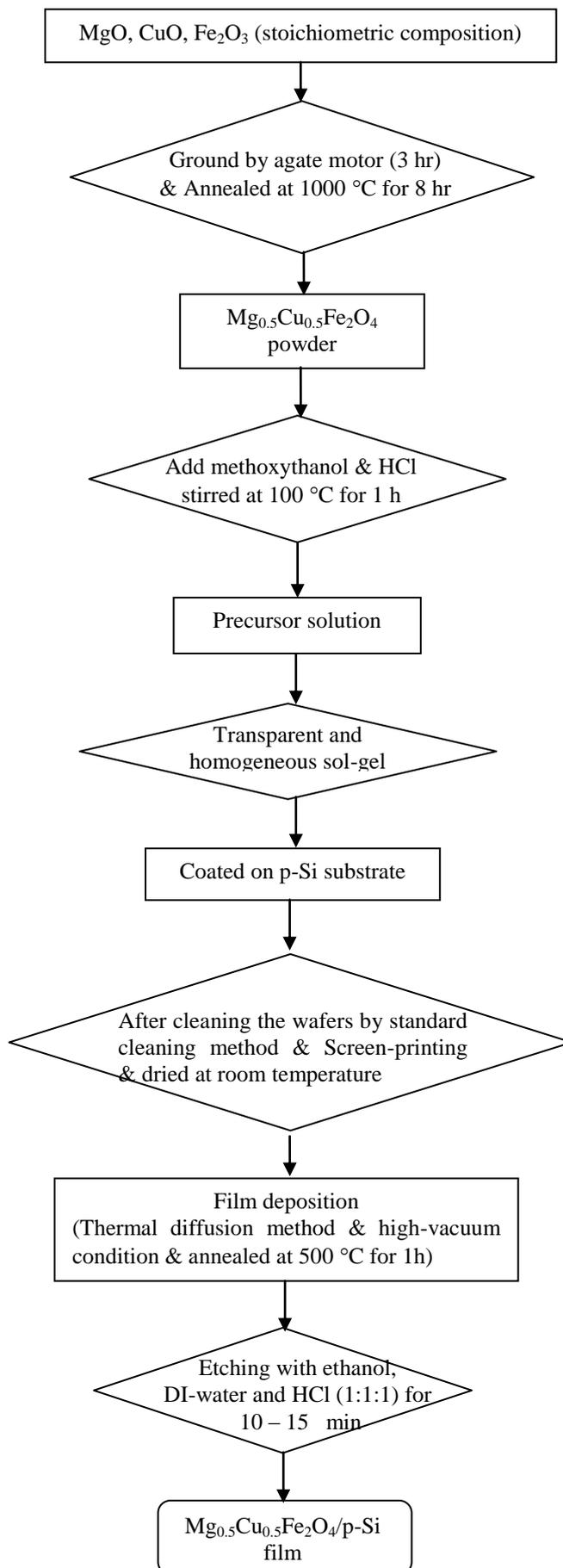
**Figure 2** Flow-diagram of the  $\text{Mg}_{0.5}\text{Cu}_{0.5}\text{Fe}_2\text{O}_4/\text{p-Si}$  thin film
