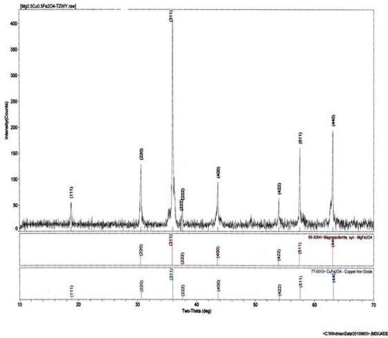
**Figure 4** XRD pattern of Magnesium-Copper mixed spinel ferrite,  $Mg_{0.5}Cu_{0.5}Fe_2O_4$
