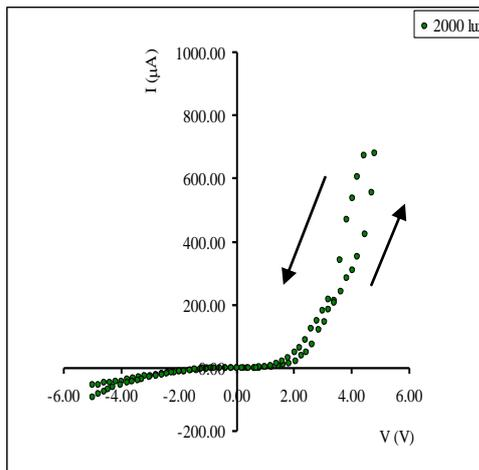
**Figure 7(f)** I-V characteristic curve of  $Mg_{0.5}Cu_{0.5}Fe_2O_4/p-Si$  thin film in 2000 lux illumination condition
