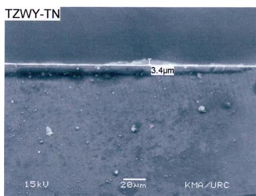
**Figure 5(c)** Diffusion layer thickness of  $\text{Mg}_{0.5}\text{Cu}_{0.5}\text{Fe}_2\text{O}_4/\text{p-Si}$  thin film
