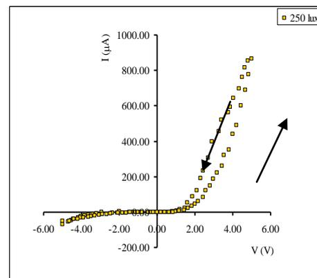
**Figure 7(b)** I-V characteristic curve of  $Mg_{0.5}Cu_{0.5}Fe_2O_4/p\text{-Si}$  thin film in ambient (250 lux) illumination condition
