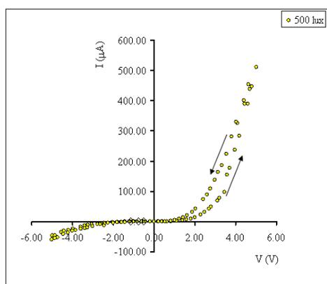
**Figure 7(c)** I-V characteristic curve of  $Mg_{0.5}Cu_{0.5}Fe_2O_4/p\text{-Si}$  thin film in 500 lux illumination condition
