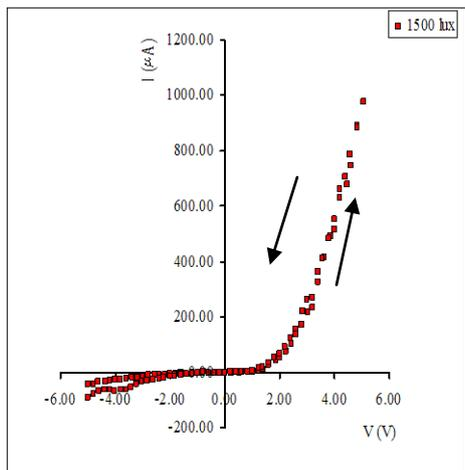
**Figure 7(e)** I-V characteristic curve of  $Mg_{0.5}Cu_{0.5}Fe_2O_4/p-Si$  thin film in 1500 lux illumination condition
