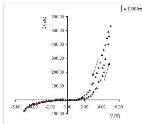
**Figure 7(d)** I-V characteristic curve of  $Mg_{0.5}Cu_{0.5}Fe_2O_4/p\text{-Si}$  thin film in 1000 lux illumination condition
