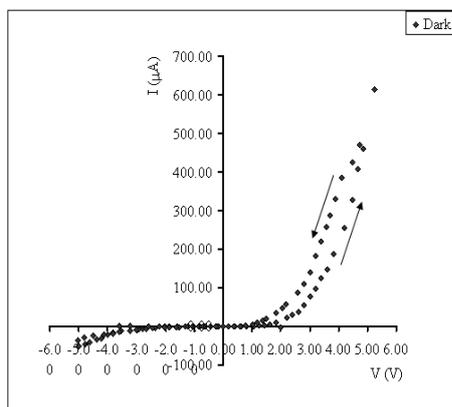
**Figure 7(a)** I-V characteristic curve of  $Mg_{0.5}Cu_{0.5}Fe_2O_4/p\text{-Si}$  thin film in dark (0 lux) condition
