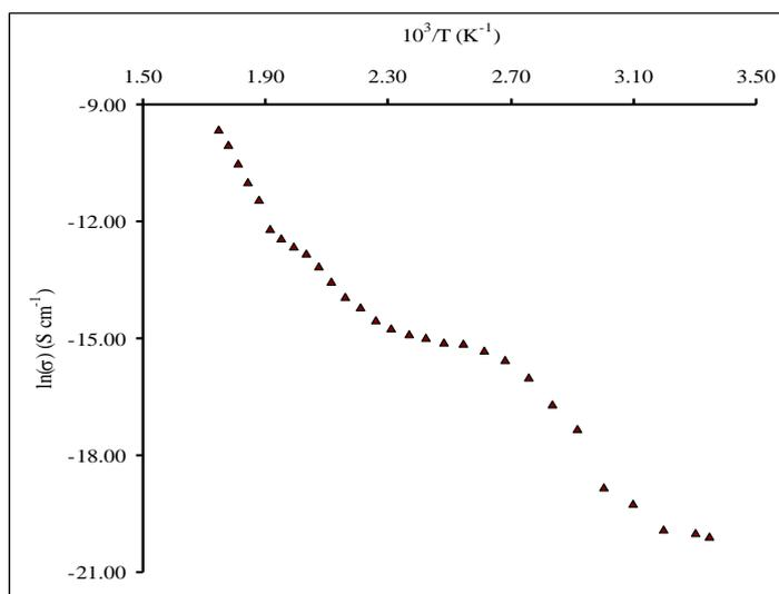
**Figure 6** Arrhenius plot of the temperature dependent electrical conductivity of  $\text{Mg}_{0.5}\text{Cu}_{0.5}\text{Fe}_2\text{O}_4$  mixed spinel ferrite
