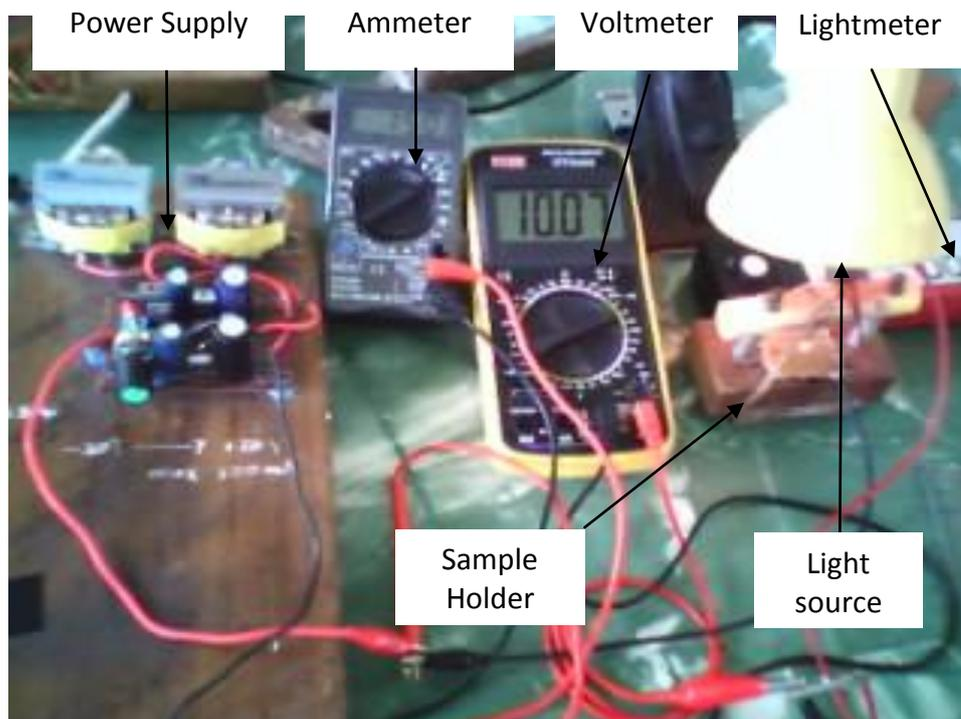
**Figure 3** Photograph of the experimental arrangement of I-V characteristic measurement
