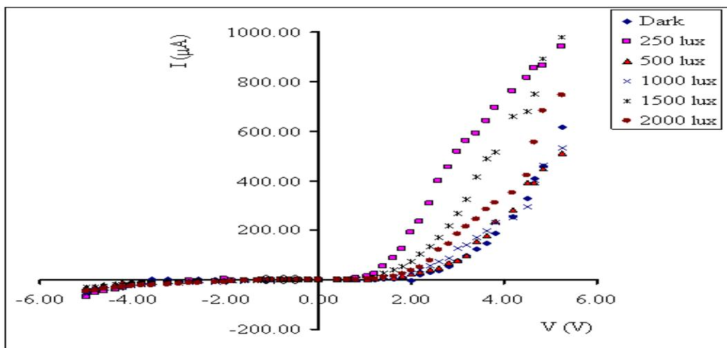
**Figure 7(g)** Comparison of the I-V characteristic curve of  $Mg_{0.5}Cu_{0.5}Fe_2O_4/ p-Si$  film in dark and in different illumination condition
