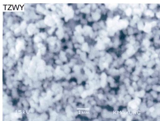
**Figure 5(b)** SEM image of  $\text{Mg}_{0.5}\text{Cu}_{0.5}\text{Fe}_2\text{O}_4/\text{p-Si}$  thin film
