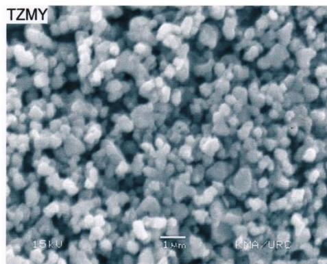
**Figure 5(a).** SEM image of Magnesium-copper mixed spinel ferrite,  $Mg_{0.5}Cu_{0.5}Fe_2O_4$  powder
