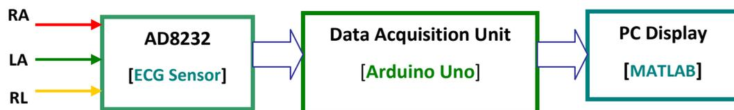
**Figure 1** Typical ECG Measurement System
