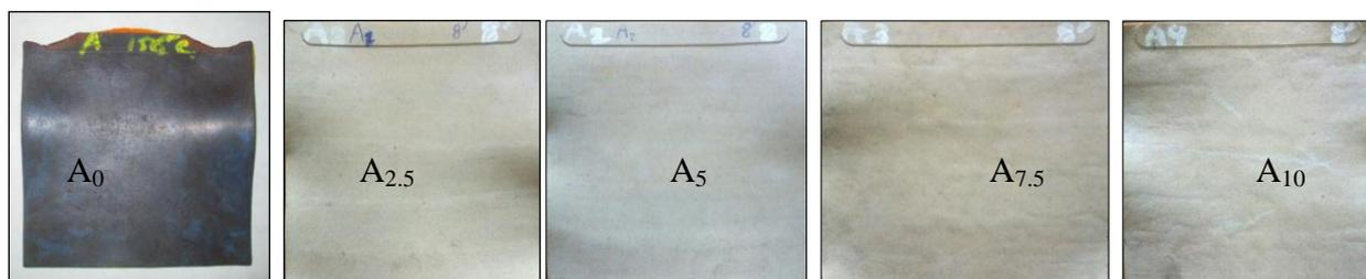
**Figure 1** Natural rubber chitosan composites A<sub>0</sub>, A<sub>2.5</sub>, A<sub>5</sub>, A<sub>7.5</sub> and A<sub>10</sub>
