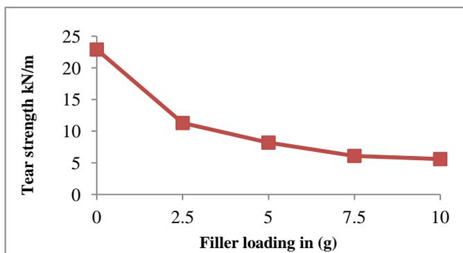
**Figure 6** Tear strength of the prepared natural rubber chitosan composites (A<sub>0</sub>-A<sub>10</sub>)
