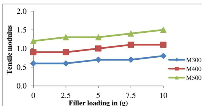
**Figure 5** Tensile modulus of the prepared natural rubber chitosan composites (A<sub>0</sub>-A<sub>10</sub>)
