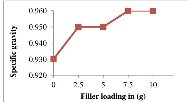
**Figure 2** Specific gravity of the prepared natural rubber chitosan composites (A<sub>0</sub>-A<sub>10</sub>)
