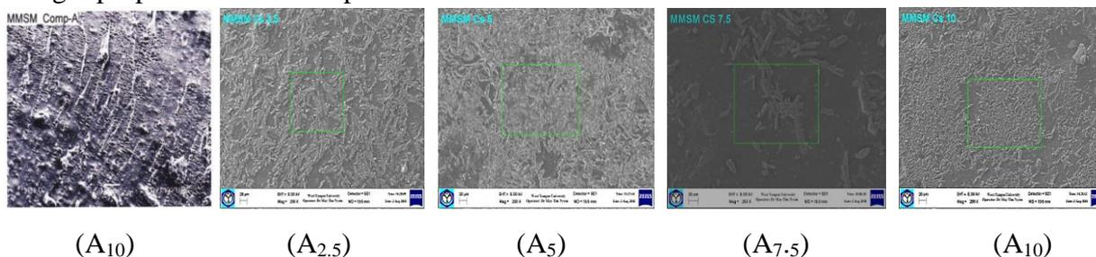
**Figure 7** Scanning electron micrographs of the prepared natural rubber chitosan composites (A<sub>0</sub>-A<sub>10</sub>)
