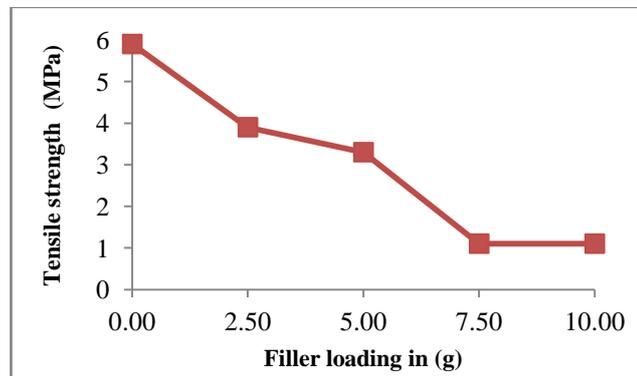
**Figure 3** Tensile strength of the prepared natural rubber chitosan composites (A<sub>0</sub>-A<sub>10</sub>)
