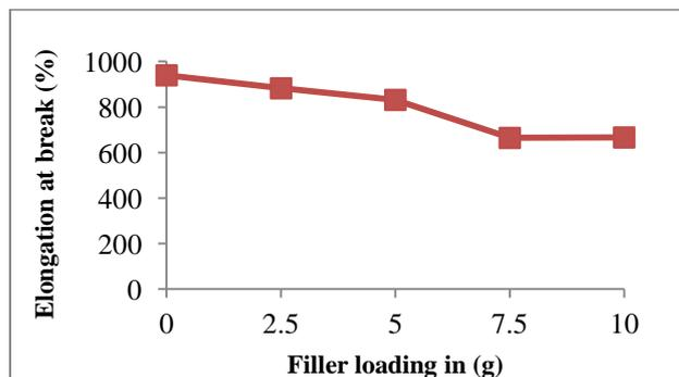
**Figure 4** Elongation at break of the prepared natural rubber chitosan composites (A<sub>0</sub>-A<sub>10</sub>)
