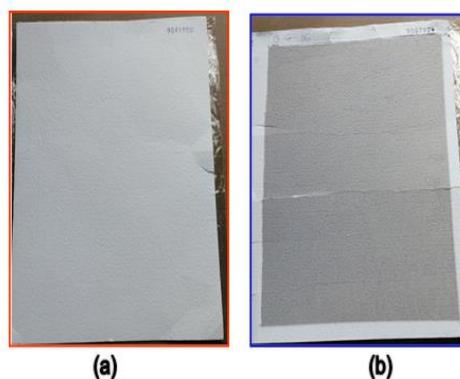
**Figure 3:** Filter papers (a) Unloaded filter paper and (b) loaded filter paper
