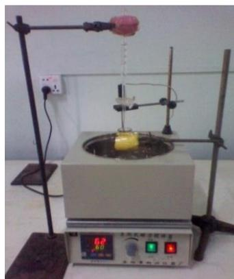
**Figure 1:** Experimental setup for synthesis of ZnO nanoparticles.
