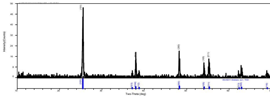
**Figure 4(a).** XRD patterns of undoped TiO<sub>2</sub> powder at 800°C
