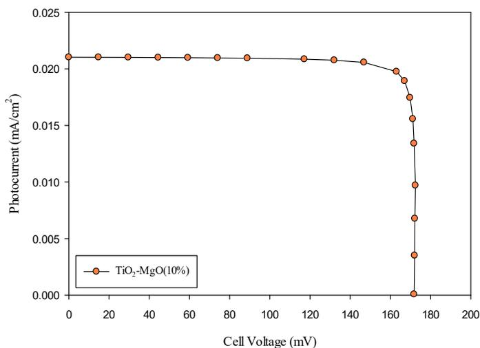
**Figure 7(c).** Current voltage characteristic curve of TiO<sub>2</sub> (90%)-MgO(10%) cell
