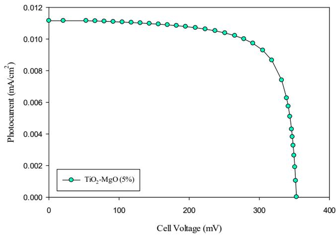
**Figure 7(b).** Current voltage characteristic curve of TiO<sub>2</sub>(95%)-MgO(5%) cell
