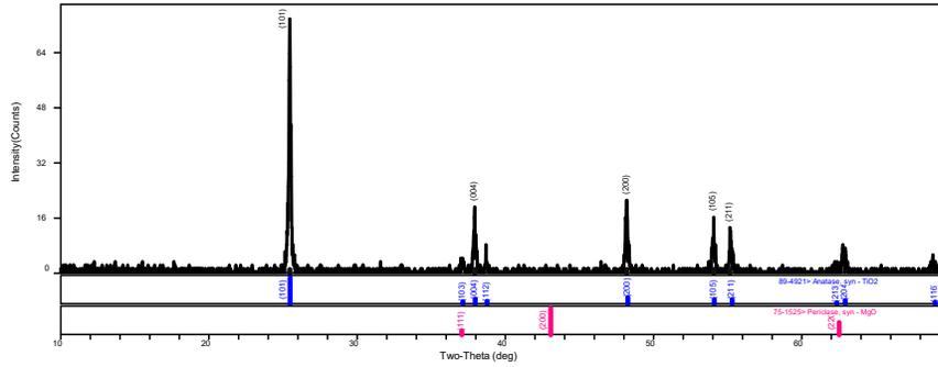
Figure 4(c). XRD patterns of TiO<sub>2</sub>(90%)-MgO(10%) at 800°C
