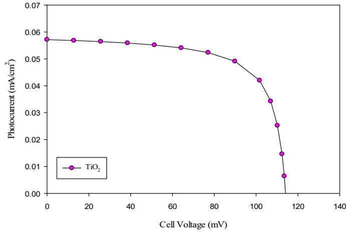
**Figure 7(a).** Current voltage characteristic curve of undoped TiO<sub>2</sub> cell
