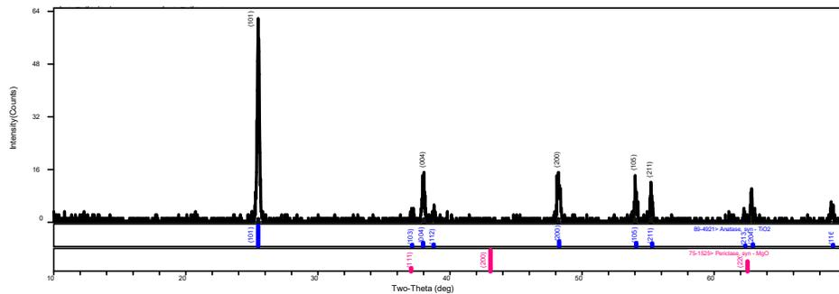
**Figure 4(b. )** XRD patterns of TiO<sub>2</sub>(95%) –MgO(5%) at 800°C
