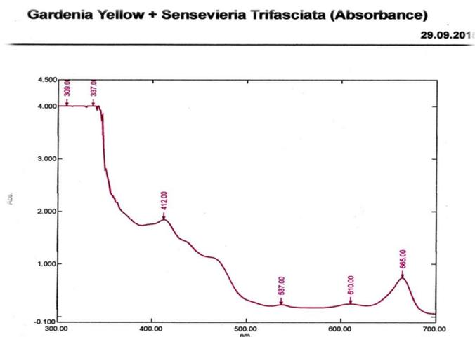
**Figure 6.** UV-Vis absorbance spectra of mixed dye solution with ethanol
