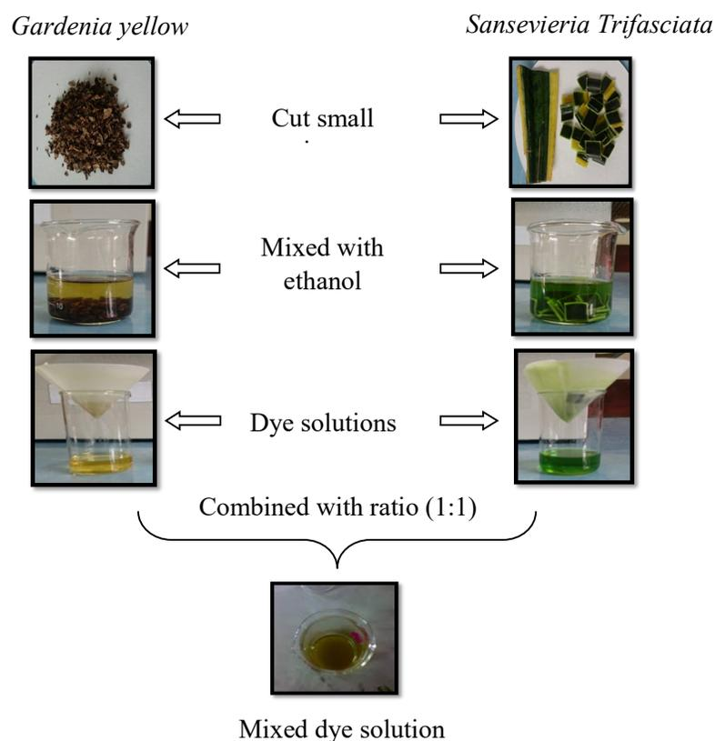
**Figure 1.** Process of dye solution preparation
