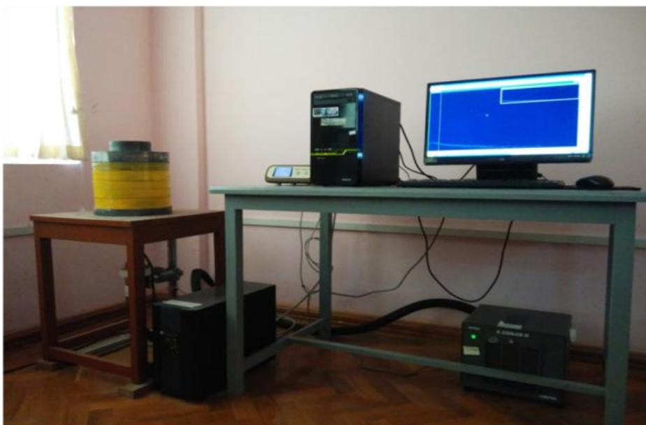
**Figure 3** The photograph of HPGe detector
