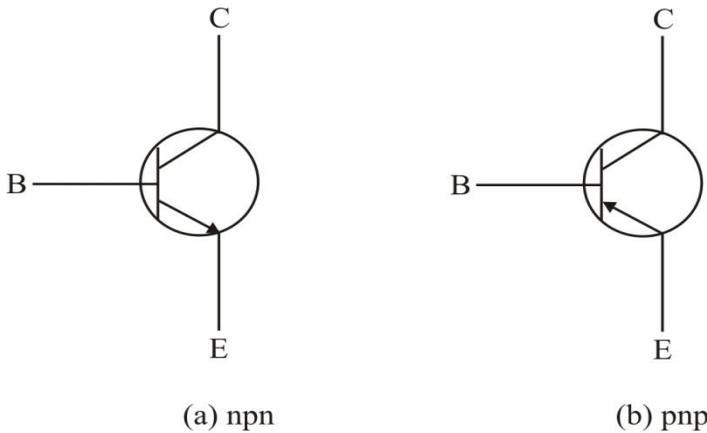
**Figure 2:** Standard bipolar junction transistor (BJT) symbols
