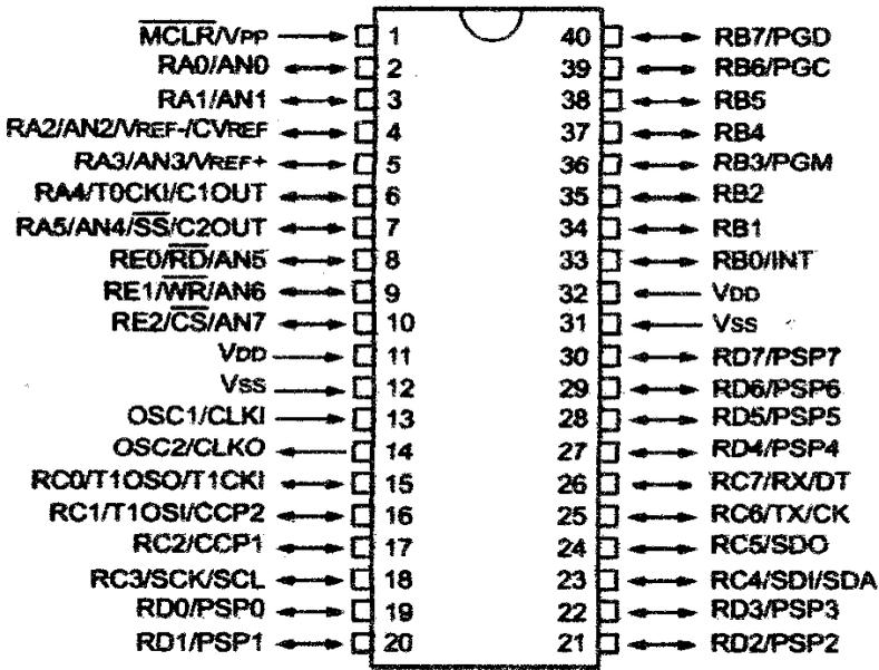
**Figure 1:** Pin diagram of PIC16F877A microcontroller
