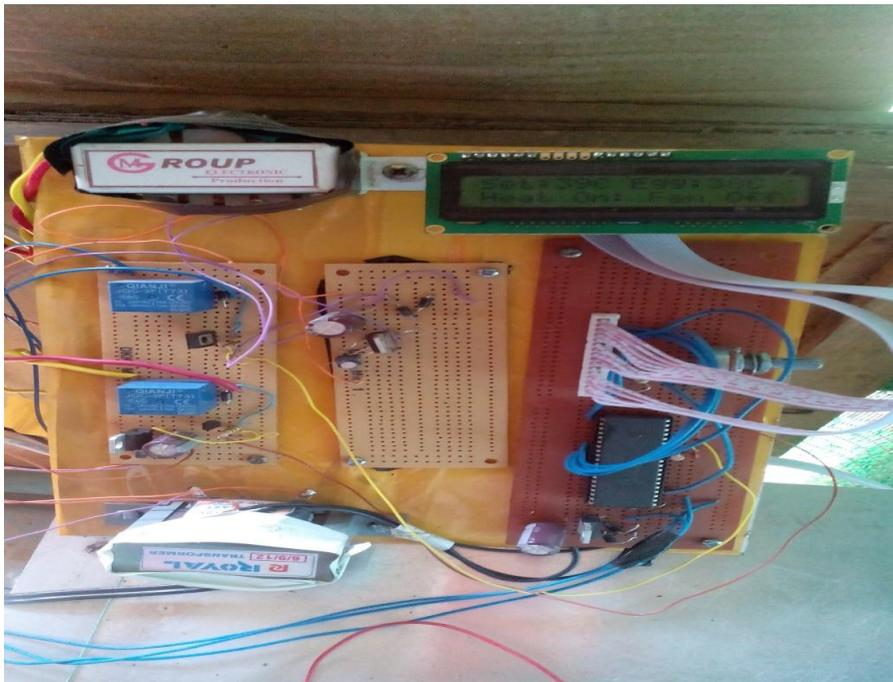
**Figure 8:** Photograph of the controlled circuit for hen egg incubator.
