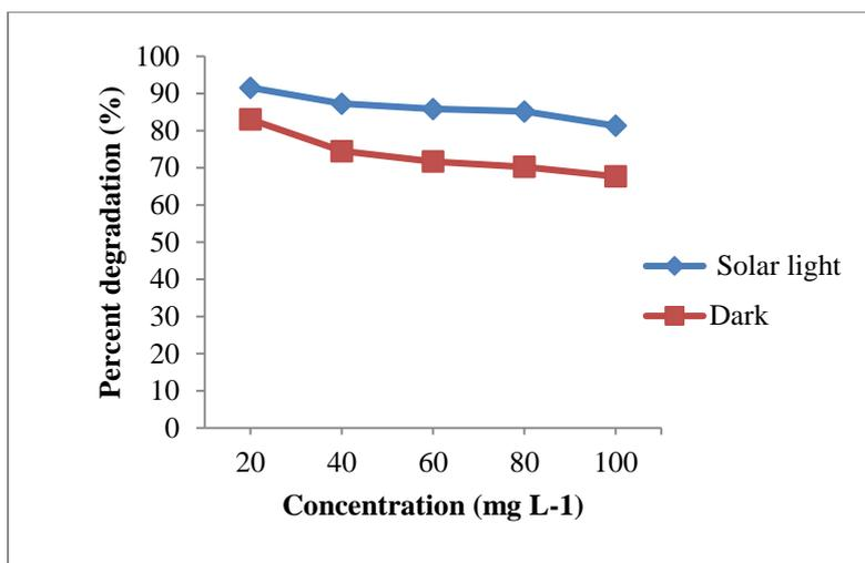
**Figure 4.** The percent degradation of MB by HA-cemented TiO<sub>2</sub> composite at different initial concentrations (solar light and dark)
