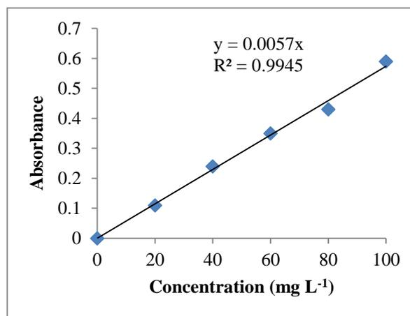
**Figure 3.** Calibration curve for methylene blue solution
