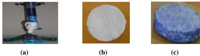
**Figure 2.** Photographs of (a) experimental filtration unit for the degradation of the methylene blue (b) methylene blue before and (c) after sorbed on HA-cemented TiO<sub>2</sub> composite
