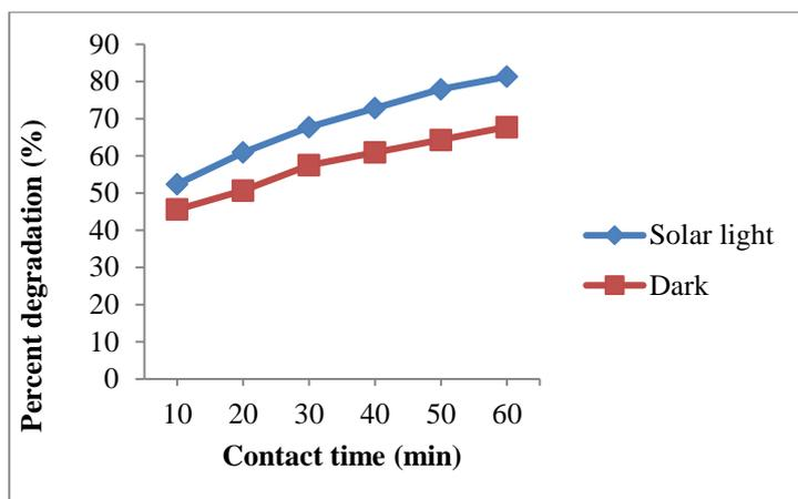
**Figure 5.** The percent degradation of MB in solar light and dark by HA-cemented TiO<sub>2</sub> composite at different contact times
