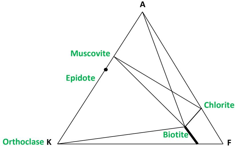
**Figure 4** AKF diagram showing the mineral assemblages of Greenschist facies (after Turner and Verhoogen, 1960)
