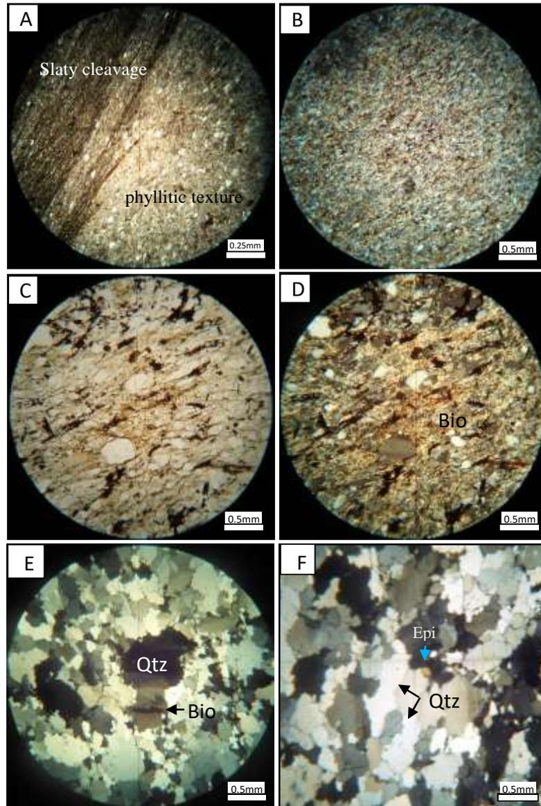
**Figure 3** (A) Slaty cleavage and phyllitic texture (under PPL and between X.N, 10X)
