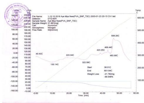
Figure 11 TG-DTA thermogram of PVA-SNP-3 film
