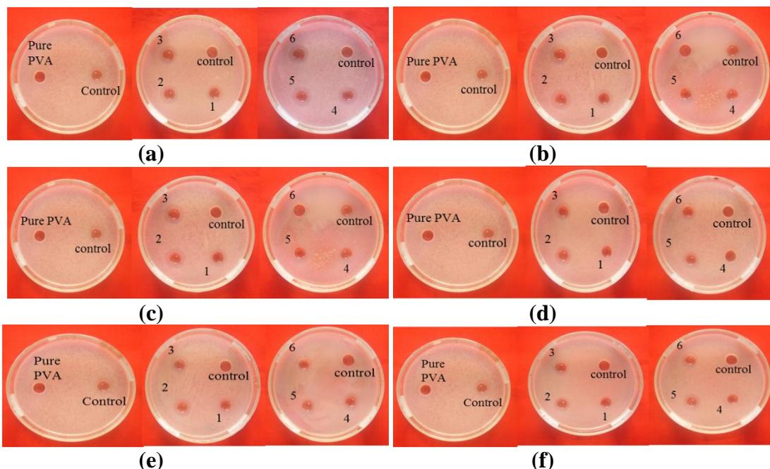
**Figure 13** Antimicrobial activity of the prepared (1) PVA-SNP-1, (2) PVA-SNP-2, (3) PVA-SNP-3, (4) PVA-SNP-4, (5) PVA-SNP-5 and (6) PVA-SNP-6 composite films
