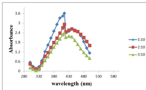
**Figure 2** Wavelength of maximum absorption of the prepared silver nanoparticles (SNP-TSC) by chemical method
