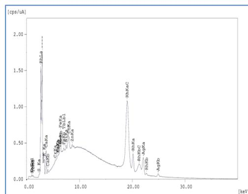
Figure 12 EDXRF spectrum of PVA-SNP-3 film
