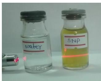
**Figure 1** Tyndall effect on the prepared SNPs by chemical synthesis
