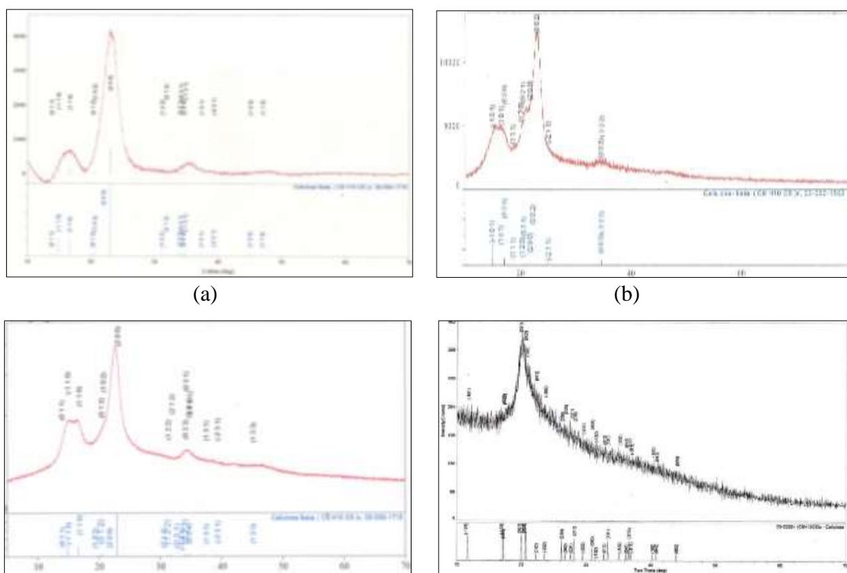
**Figure 1** XRD diffractograms of (a) raw pineapple leaf fibres RPALF (b) bleached pineapple leaf fibres BPALF (c) cellulose pineapple leaf fibres CPALF and (d) carboxymethyl cellulose CMC
