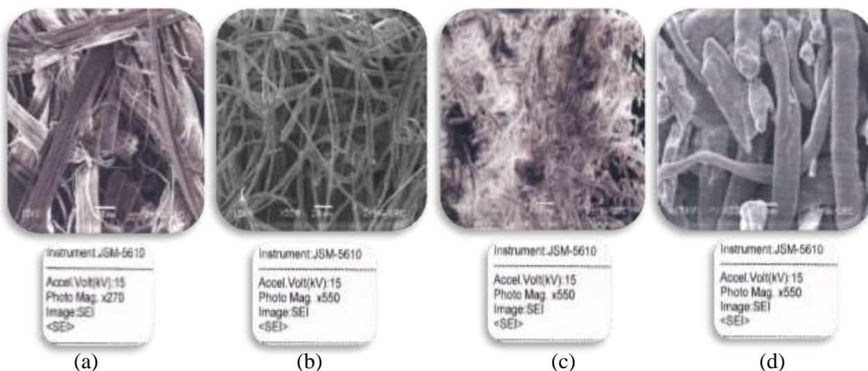
**Figure 3** SEM micrographs of (a) raw pineapple leaf fibres RPALF (b) bleached pineapple leaf fibres BPALF (c) cellulose pineapple leaf fibres CPALF and (d) carboxymethyl cellulose CMC
