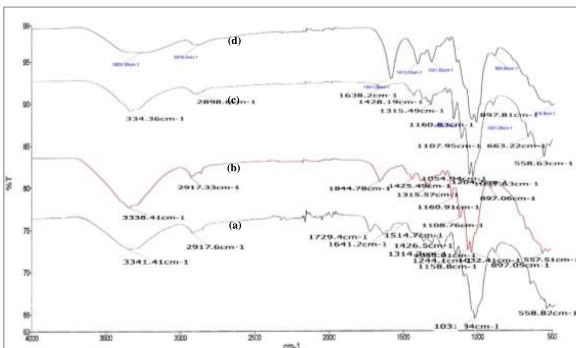
**Figure 2** FT IR spectra of (a) raw pineapple leaf fibres RPALF (b) bleached pineapple leaf fibres BPALF (c) cellulose pineapple leaf fibres CPALF and (d) carboxymethyl cellulose CMC
