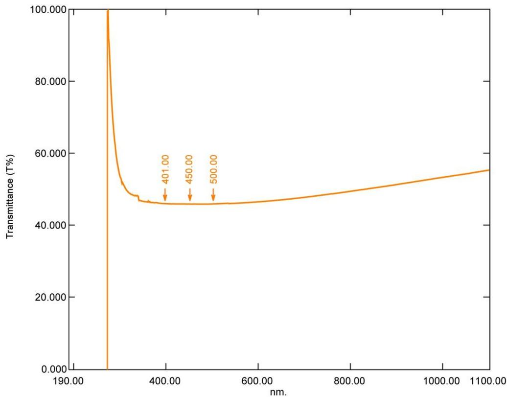
**Figure 2 (e)** Transmittance (T%) spectra for Sb (8 mol%) doped SnO<sub>2</sub> thin film on glass
