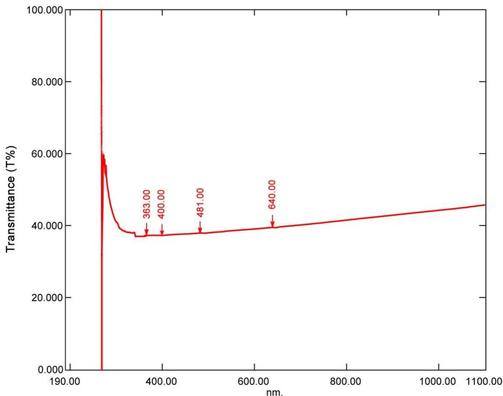
**Figure 2 (d)** Transmittance (T%) spectra for Sb (6 mol%) doped SnO<sub>2</sub> thin film on glass
