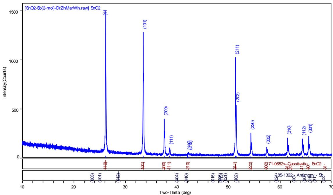
Figure 1 (b) XRD pattern of Sb (2 mol%) doped SnO<sub>2</sub> thin film on glass
