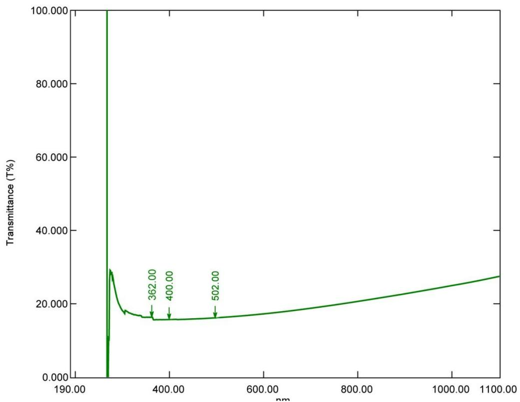
Figure 2 (c) Transmittance (T%) spectra for Sb (4 mol%) doped SnO<sub>2</sub> thin film on glass
