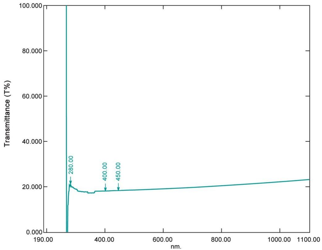
Figure 2 (b) Transmittance (T%) spectra for Sb (2 mol%) doped SnO<sub>2</sub> thin film on glass
