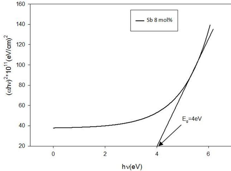
**Figure 3 (e)** Plot of  $(\alpha hv)^2$  versus  $hv$  (Sb 8 mol% doped)
