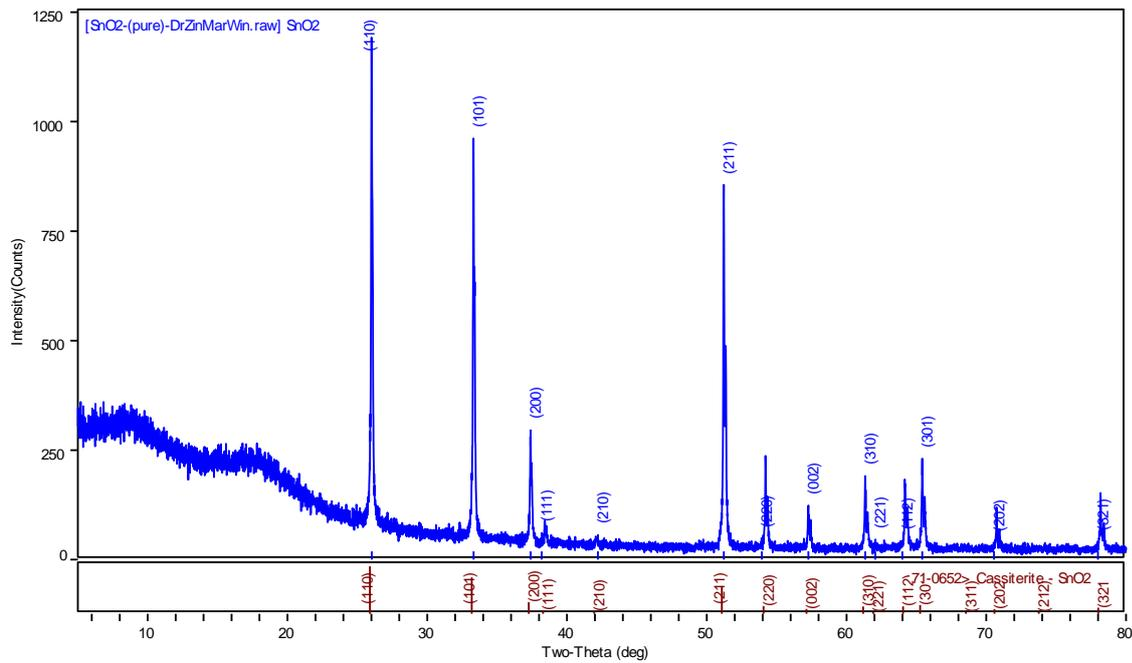
Figure 1 (a) XRD pattern of undoped SnO<sub>2</sub> thin film on glass
