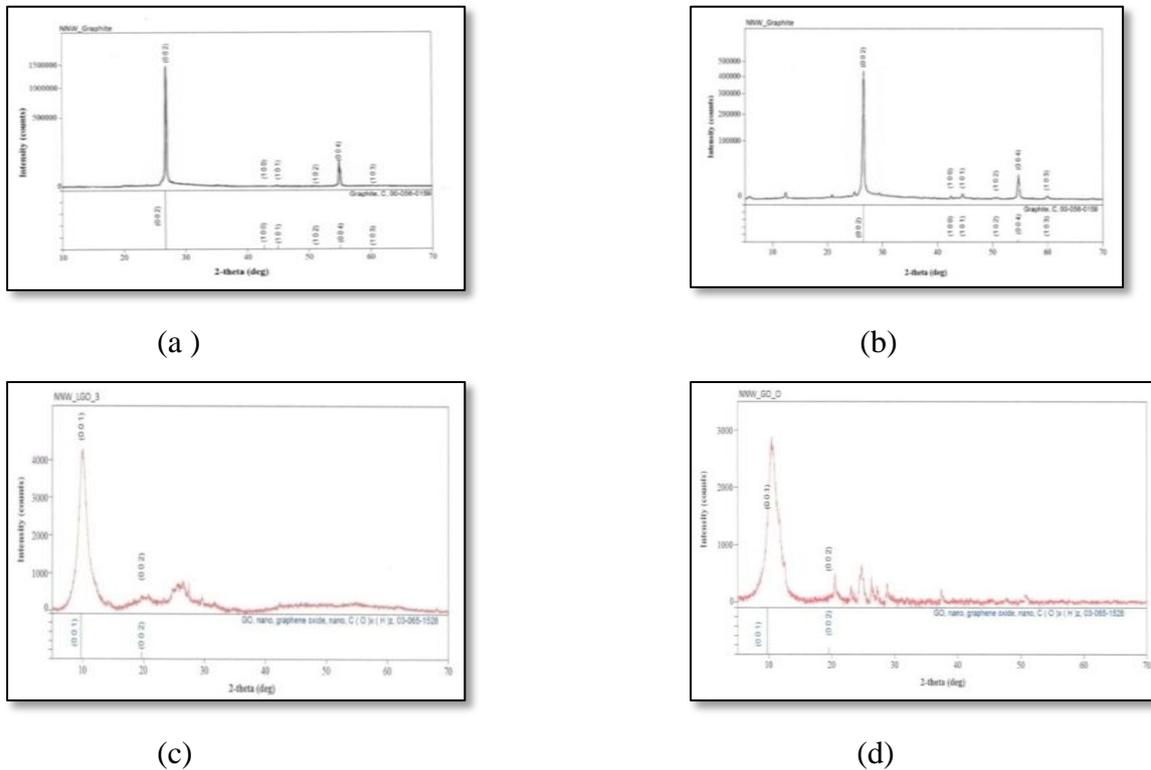
**Figure 1** XRD diffractograms of (a) local mine graphite (LGP) (b) commercial graphite (CGP) (c) prepared graphene oxide (LGO) and (d) prepared graphene oxide (CGO)
