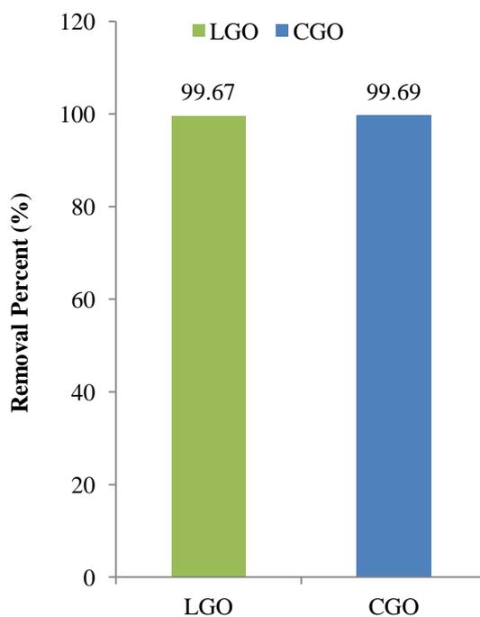
**Figure 11** Comparison of removal percent of methylene blue solution under optimal condition
