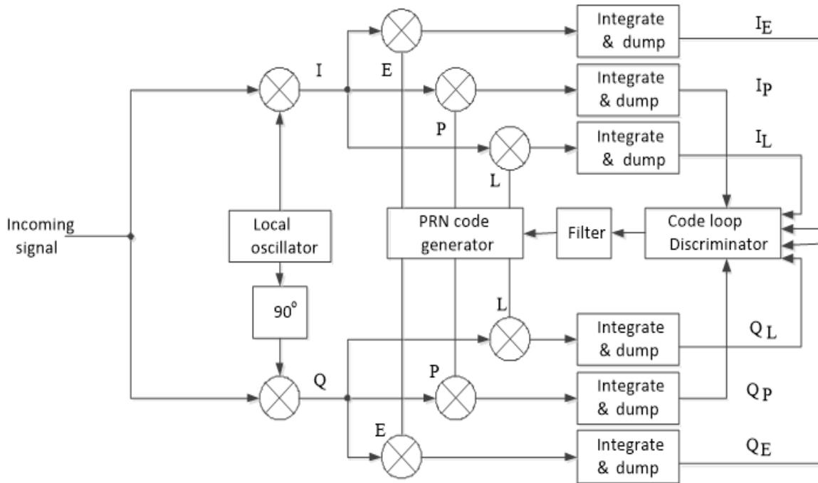
Figure 2 Delay Lock Loop (DLL) block diagram with six correlators
