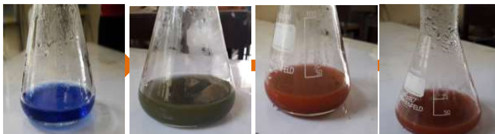
Figure. 1. Color changes (blue , green, red to dark brown) of solution after mixing NaOH 2.5 M \text{CuNO}_3 of 0.5 M
