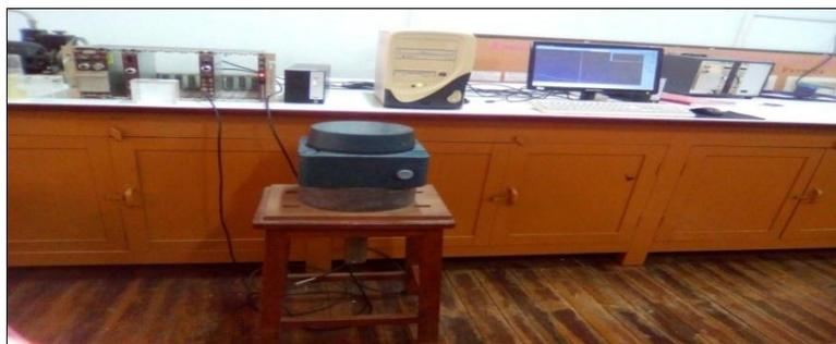
**Figure 4** The measurement arrangement with the NaI(Tl) detector
