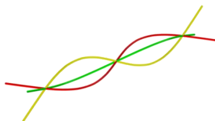
Figure 4 Second mode at eigenfrequency 457.85 Hz
