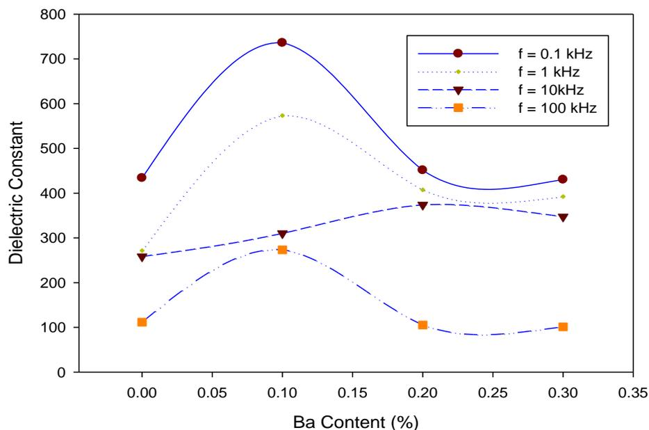
**Figure 3** (b) The dependence of dielectric constant of the  $\text{CaTiO}_3$  thin films on the Ba content
