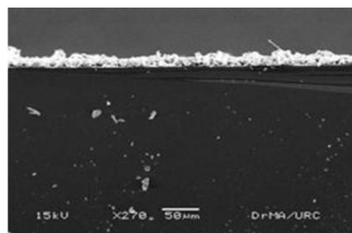
**Figure 1 (f)** Cross sectional image 10% Ba doped CT thin film
