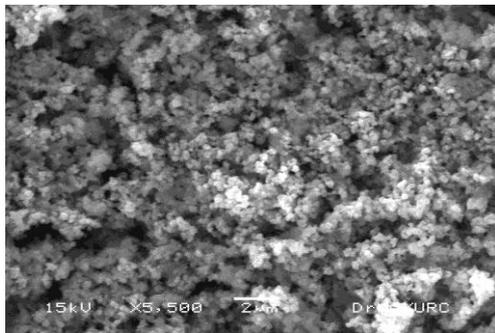
**Figure 1(c)** SEM image of 20% Ba doped CT thin film
