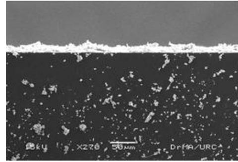
**Figure 1 (h)** Cross sectional image 30% doped CT thin film
