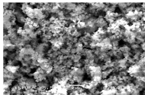
**Figure 1 (d)** SEM image of 30% Ba doped CT thin film
