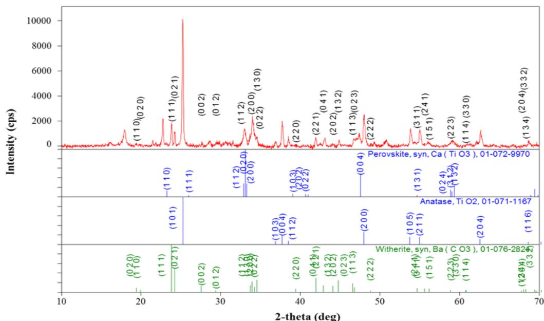
Figure 2 (d) X-ray diffraction of 30% Ba doped  $\text{CaTiO}_3$  thin film
