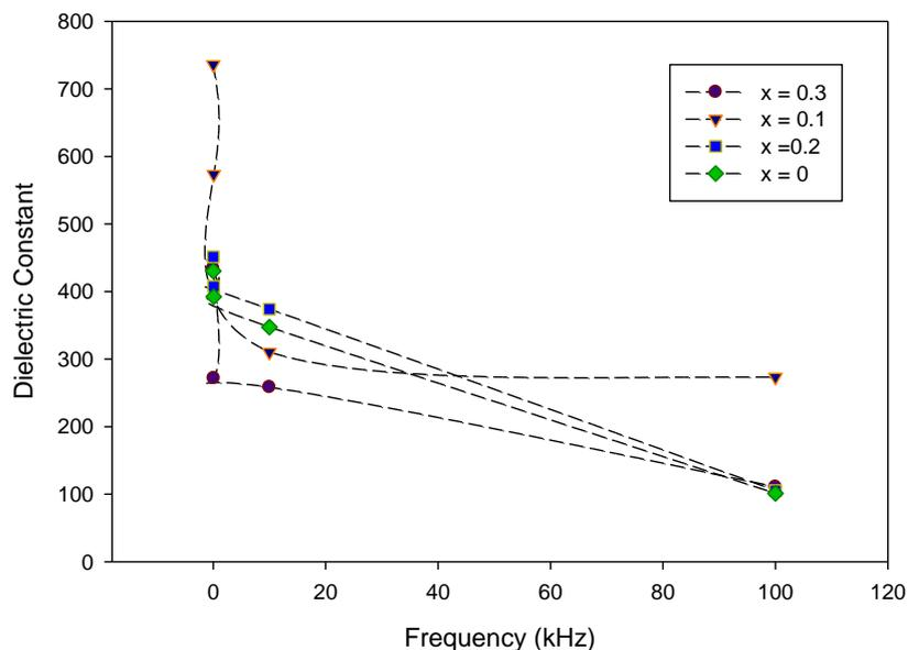
**Figure 3 (a)** The dependence of dielectric constant of the CaTiO<sub>3</sub> thin films as a function of frequency
