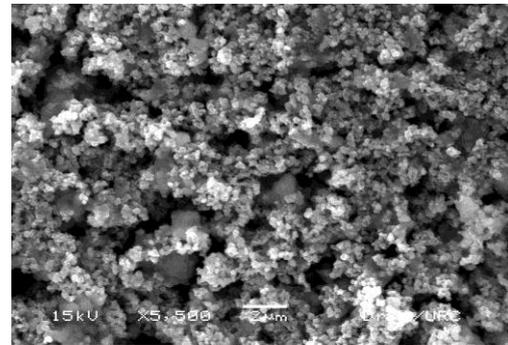
**Figure 1 (b)** SEM image of 10% Ba doped CT thin film
