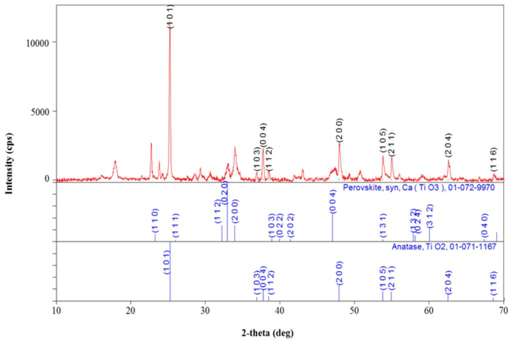
Figure 2 (c) X-ray diffraction of 20% Ba doped  $\text{CaTiO}_3$  thin film
