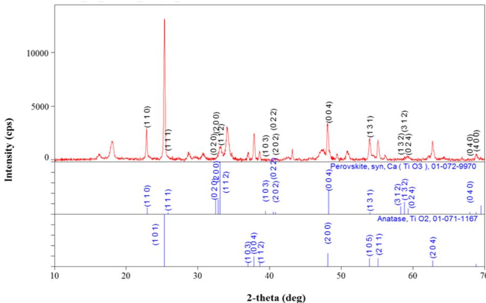
**Figure 2 (a)** X-ray diffraction of CaTiO<sub>3</sub> thin film
