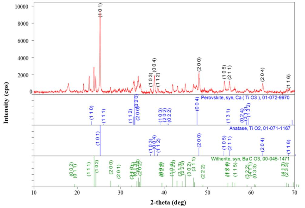
Figure 2 (b) X-ray diffraction of 10% Ba doped  $\text{CaTiO}_3$  thin film
