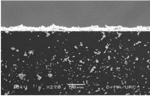
**Figure 1 (g)** Cross sectional image 20% Ba Ba doped CT thin film
