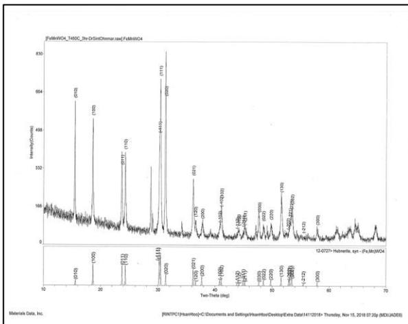
**Figure 3** XRD pattern of 70% (Fe,Mn)WO<sub>4</sub> at 450 °C in three hours
