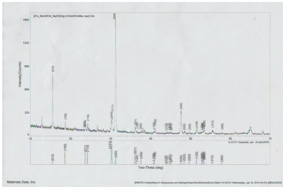
Figure 6 XRD pattern of natural wolframite powder samples with sodium hydroxide solution
