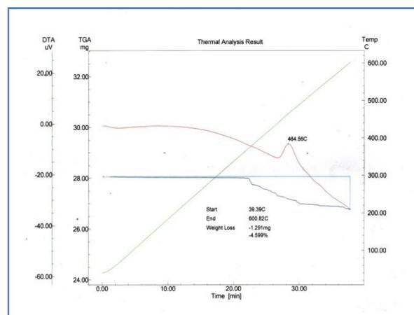
**Figure 2** TGA and TD curve of the  $(\text{Fe,Mn})\text{WO}_4$
