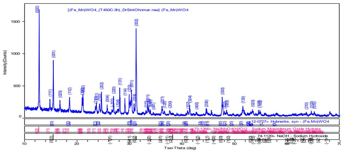
Figure 7 XRD pattern of natural wolframite powder samples with sodium hydroxide solution at 450 °C in one hours
