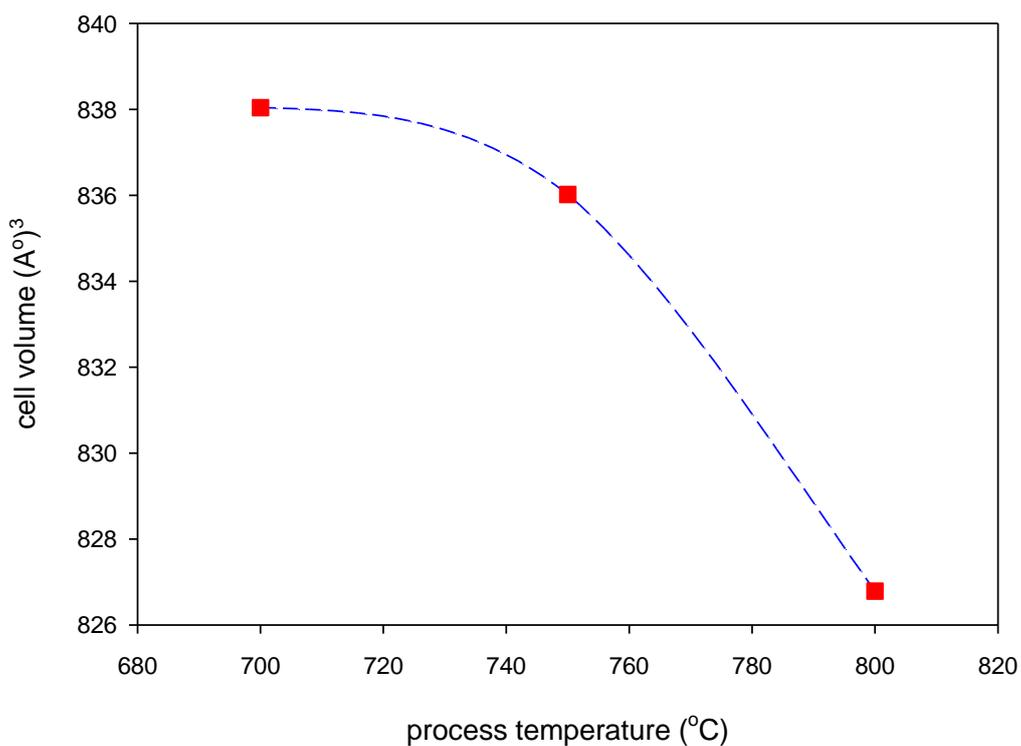
**Figure 4** The variation of process temperature with cell volume of the  $\text{Pb}_2\text{MnO}_4$  ceramics
