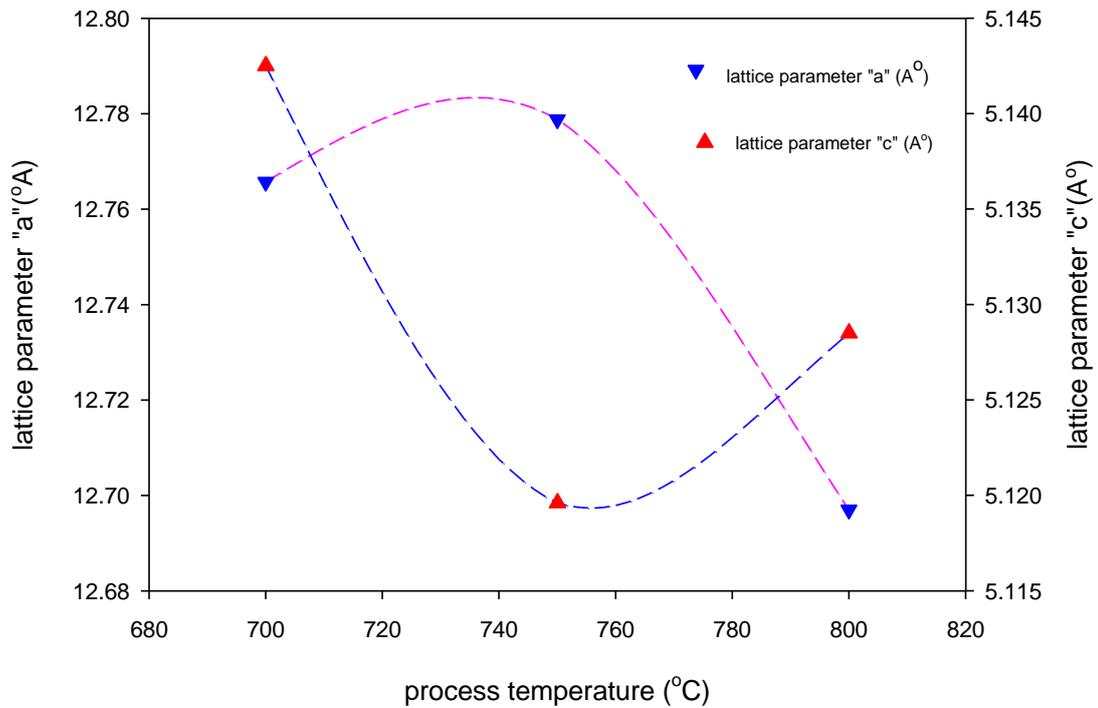
Figure 2 The variation of lattice parameters " a " and " c " with process temperature of the  $Pb_2MnO_4$  ceramics
