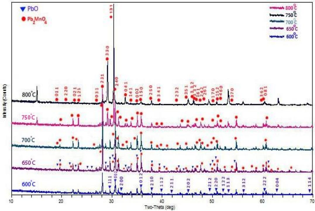
Figure 1 XRD spectra of  $Pb_2MnO_4$  ceramics at different sintering temperatures.
