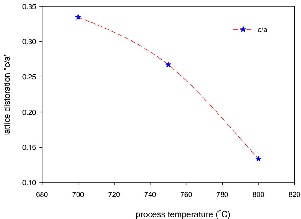
**Figure 3** The variation of process temperature with lattice distortion (c/a) of the  $\text{Pb}_2\text{MnO}_4$  ceramics
