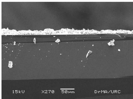
**Figure 1 (g)** Cross sectional image 30% Sr doped CTO thin film
