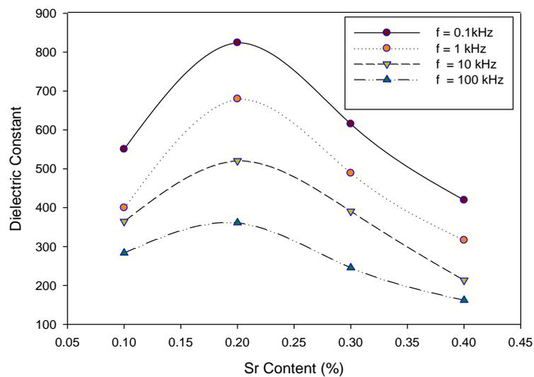
**Figure 3 (b)** The dependence of dielectric constant of the  $\text{CaTiO}_3$  thin films on the Sr content
