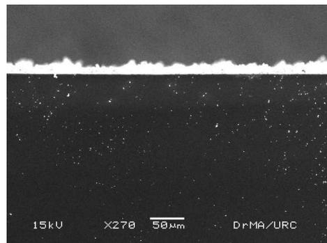
**Figure 1 (h)** Cross sectional image 40% Sr doped CTO thin film
