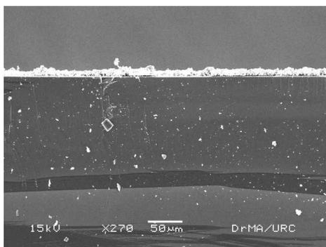
**Figure 1 (e)** Cross sectional image 10% Sr doped CTO thin film
