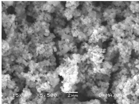
**Figure 1 (a)** SEM image of 10% Sr doped CTO thin film
