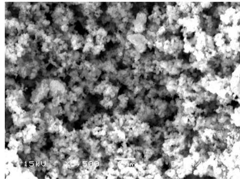
**Figure 1 (b)** SEM image of 20% Sr doped CTO thin film
