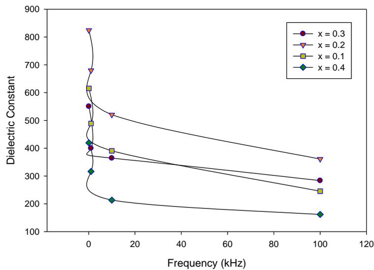
**Figure 3 (a)** The dependence of dielectric constant of the Sr doped  $\text{CaTiO}_3$  thin films as a function of frequency
