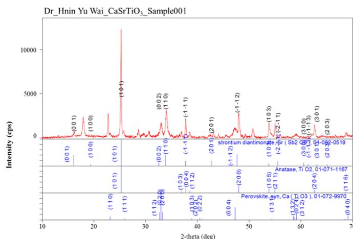
Figure 2 (a) X-ray diffraction of 10% Sr doped  $\text{CaTiO}_3$  thin film
