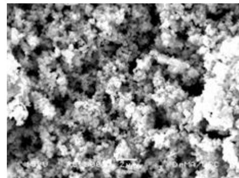
**Figure 1 (d)** SEM image of 10% Sr doped CTO thin film
