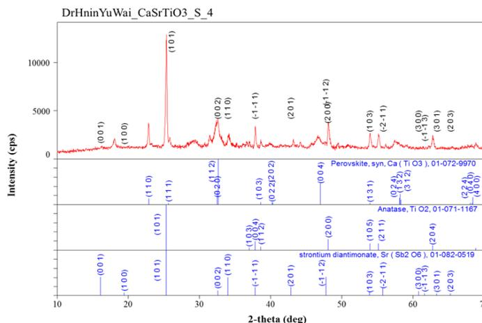
Figure 2 (d) X-ray diffraction of 40% Sr doped CaTiO<sub>3</sub> thin film
