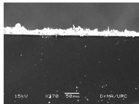
**Figure 1 (f)** Cross sectional image 20% Sr doped CTO thin film
