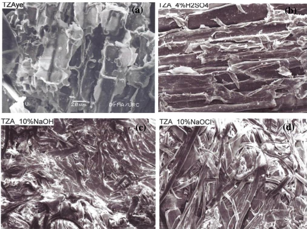
**Figure 5:** SEM photographs (20μ m magnification) of (a) sugar cane bagasse raw sample (b) acid treated sample (c) base treated sample and (d) cellulose fiber
