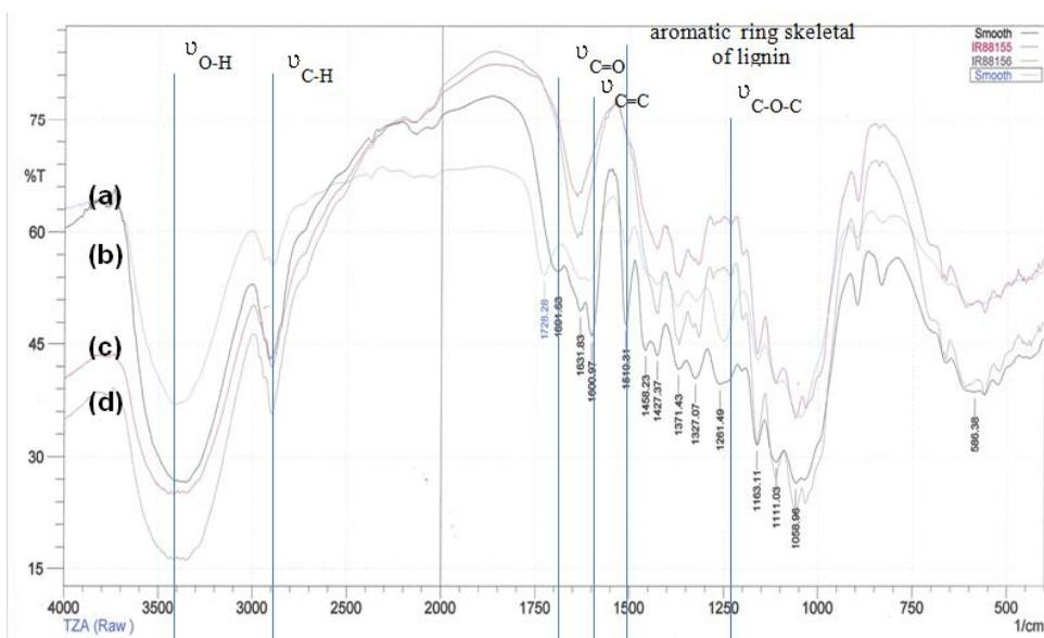
**Figure 4:** FT IR spectra of (a) sugar cane bagasse raw sample (b) acid treated sample (c) base treated sample and (d) cellulose fiber
