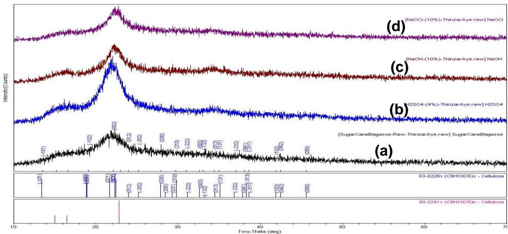
**Figure 6:** XRD patterns of (a) sugar cane bagasse raw sample (b) acid treated sample (c) base treated sample and (d) cellulose fiber
