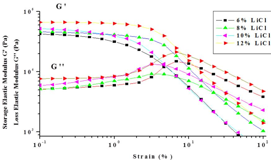
**Figure 7:** Viscoelasticity of cellulose hydrogels films of different LiCl contents for strain  $-G'$ ,  $-G''$  plots at 25 ° C
