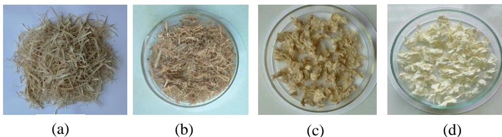
**Figure 2:** (a) Sugarcane bagasse raw sample (b) acid treated sample (c) base treated sample and (d) cellulose fiber
