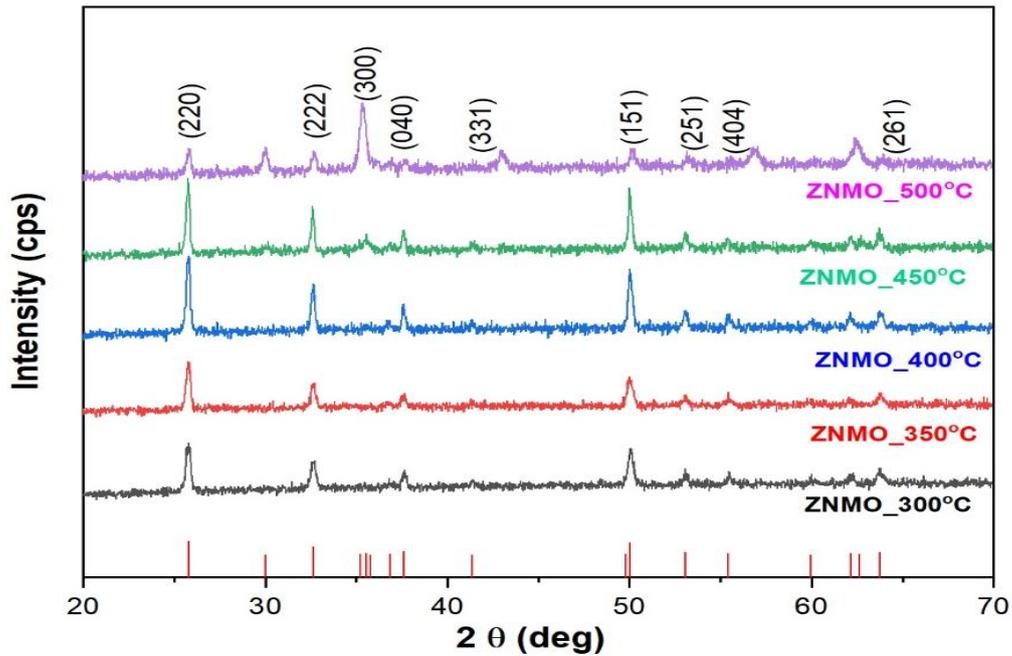
**Figure 2** The XRD patterns for Zn-Ni-Mn ternary metal oxide film on nickel foam at different temperatures
