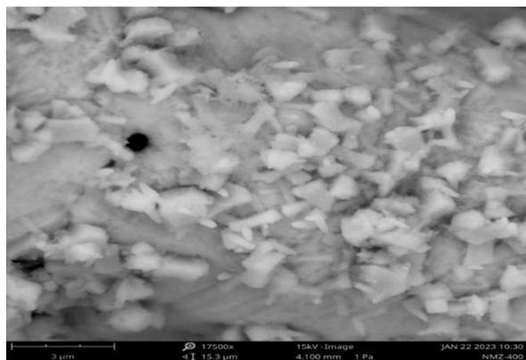
**Figure 3 (c)** SEM micrograph of Zn-Ni-Mn ternary metal oxide film at 400 °C
