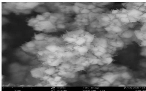
**Figure 3 (e)** SEM micrograph of Zn-Ni-Mn ternary metal oxide film at 500 °C
