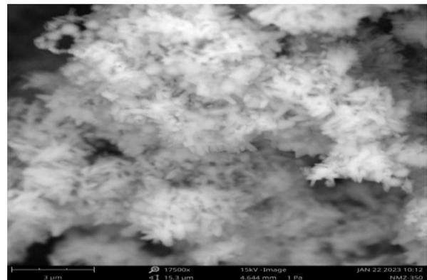
**Figure 3 (b)** SEM micrograph of Zn-Ni-Mn ternary metal oxide film at 350 °C
