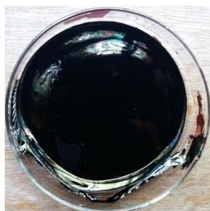
**Figure 1:** (b) Photo showing copolymer/TiO<sub>2</sub> composite film
