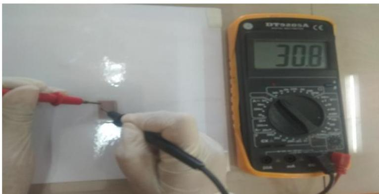
**Figure 5:** Copper nanowires ink deposited on glass substrate. Thin film of copper nanowires shows low sheet resistance 30  $\Omega$ .
