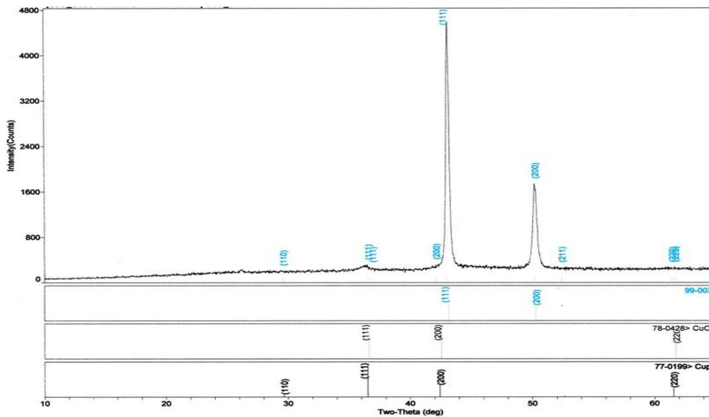
**Figure 4:** XRD plots obtained from CuNWs sample by using hydrazine 0.13 mmol to investigate the structures and crystallinity. Reference bulk reflections of pure Cu phases are shown at the bottom (ICDD-PDF#99-0034).
