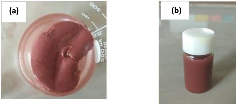
**Figure1:** Photograph of CuNWs growth solutions. (a) before and (b) after centrifugation
