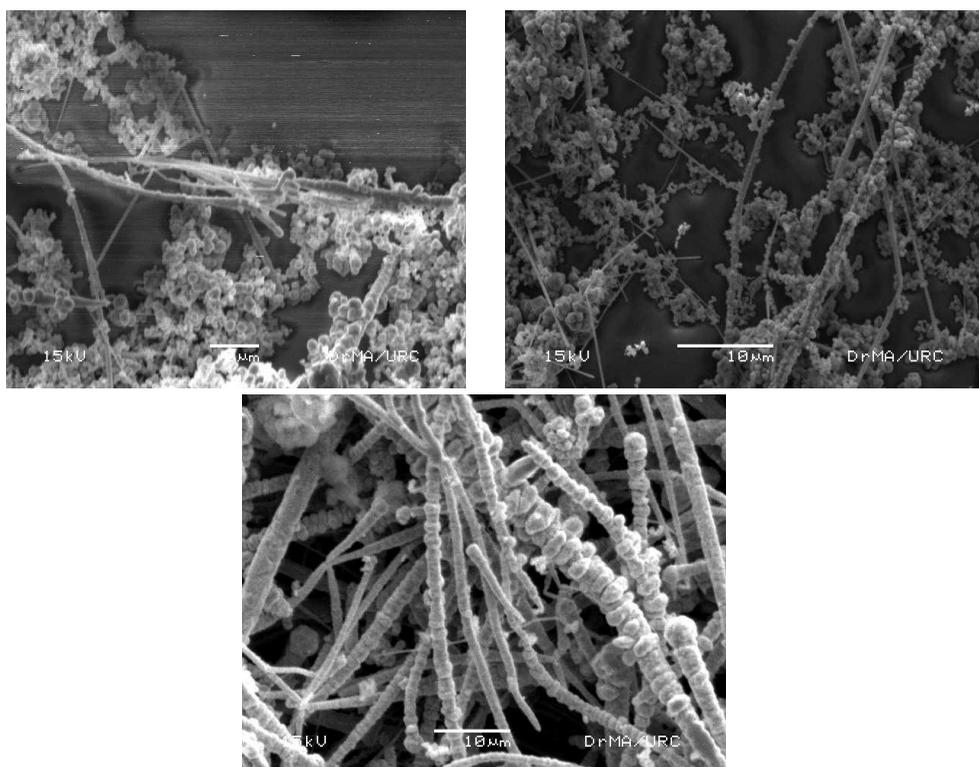
**Figure 3:** SEM micrograph of Cu Nanowires solution by using ethylenediamine with different amount of hydrazine (a) 0.22 mmol (b) 0.17 mmol and (c) 0.13mmol.
