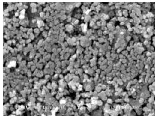
**Figure 8** SEM image of  $Mg_{(0.5)}Cu_{(0.5)}Fe_2O_4$  (800°C) sample
