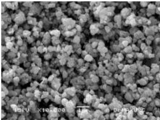
**Figure 5** SEM image of  $Mg_{(0.5)}Cu_{(0.2)}Zn_{(0.3)}Fe_2O_4$  (800°C) sample
