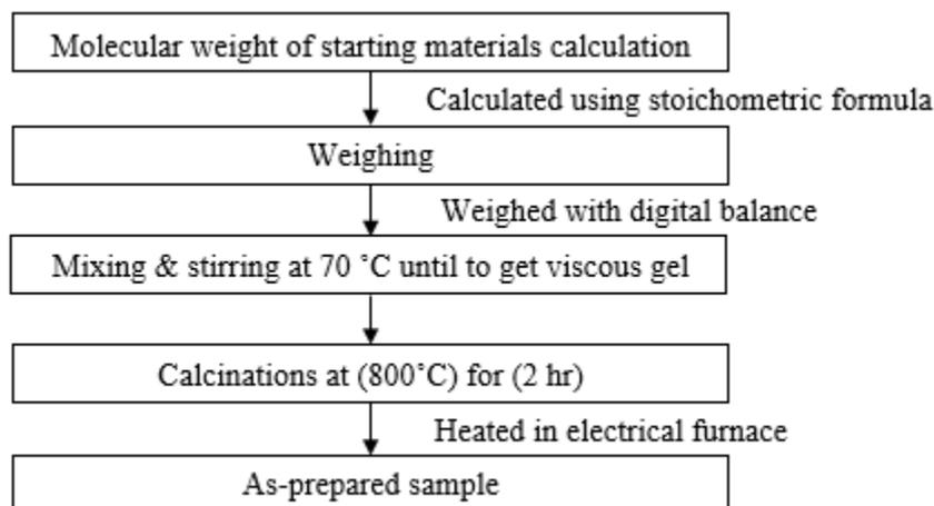
**Figure 1** Flow diagram of the sample preparation procedure of magnesium copper zinc ferrite
