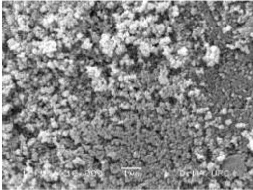
**Figure 3** SEM image of  $Mg_{(0.5)}Zn_{(0.5)}Fe_2O_4$  (800°) sample
