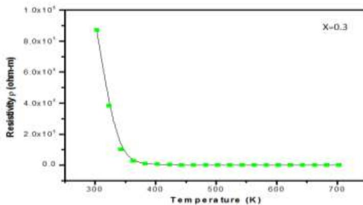
**Figure 9 (c)** Temperature dependent resistivity curves for  $\text{Mg}_{(0.5)}\text{Cu}_{(x)}\text{Zn}_{(0.5-x)}\text{Fe}_2\text{O}_4$  with Cu content ( $x=0.3$ )
