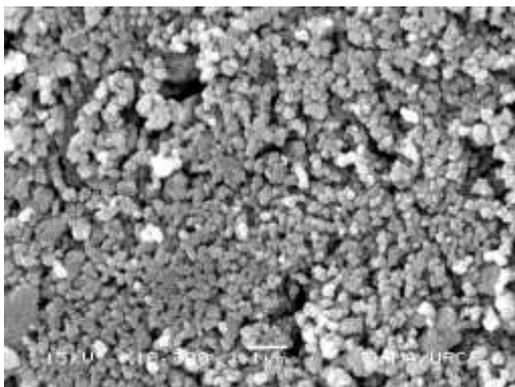
**Figure 7** SEM image of  $Mg_{(0.5)}Cu_{(0.4)}Zn_{(0.1)}Fe_2O_4$  (800°C) sample
