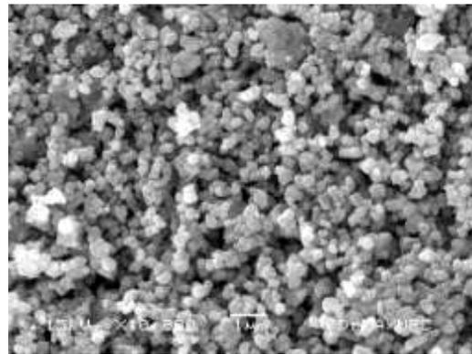
**Figure 6** SEM image of  $Mg_{(0.5)}Cu_{(0.3)}Zn_{(0.2)}Fe_2O_4$  (800°C) sample
