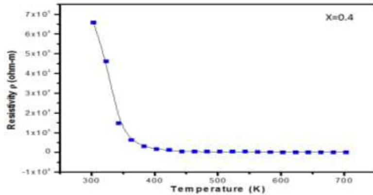
**Figure 9 (d)** Temperature dependent resistivity curves for  $Mg_{(0.5)}Cu_{(x)}Zn_{(0.5-x)}Fe_2O_4$  with Cu content ( $x=0.4$ )
