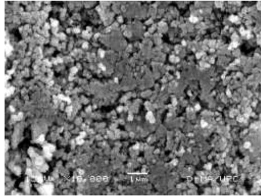
**Figure 4** SEM image of  $Mg_{(0.5)}Cu_{(0.1)}Zn_{(0.4)}Fe_2O_4$  (800°C) sample
