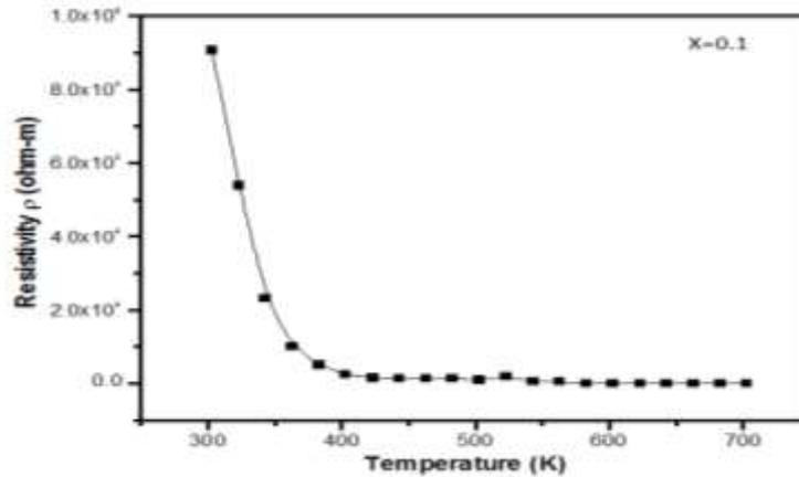
**Figure 9 (a)** Temperature dependent resistivity curves for  $\text{Mg}_{(0.5)}\text{Cu}_{(x)}\text{Zn}_{(0.5-x)}\text{Fe}_2\text{O}_4$  with Cu content ( $x=0.1$ )
