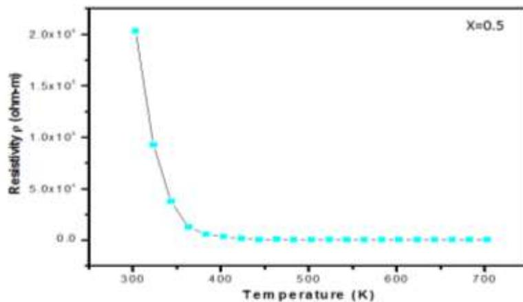
**Figure 9 (e)** Temperature dependent resistivity curves for  $Mg_{(0.5)}Cu_{(x)}Zn_{(0.5-x)}Fe_2O_4$  with Cu content ( $x=0.5$ )
