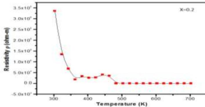
**Figure 9 (b)** Temperature dependent resistivity curves for  $\text{Mg}_{(0.5)}\text{Cu}_{(x)}\text{Zn}_{(0.5-x)}\text{Fe}_2\text{O}_4$  with Cu content ( $x=0.2$ )
